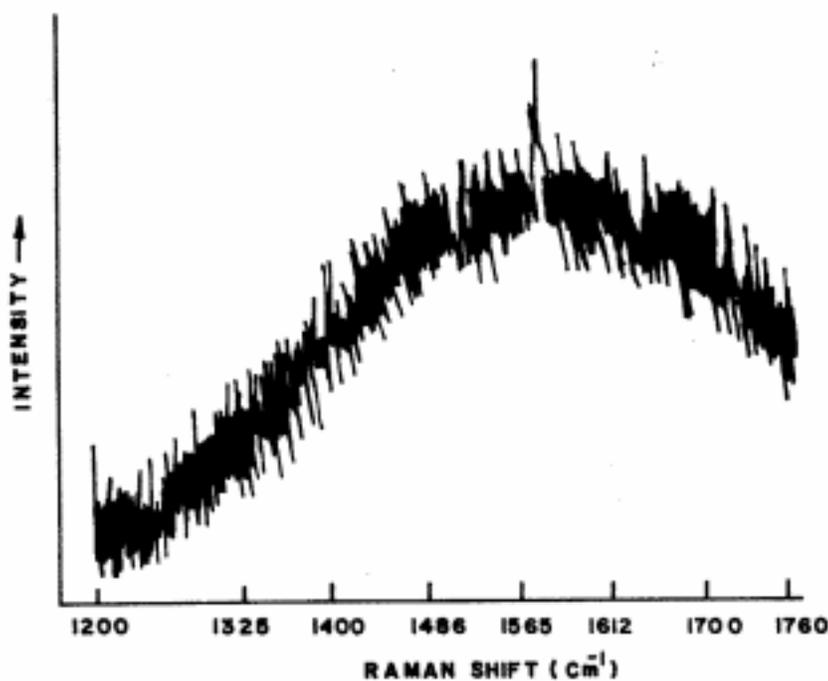
Figure 2. Raman spectra of DLC on s.s.
