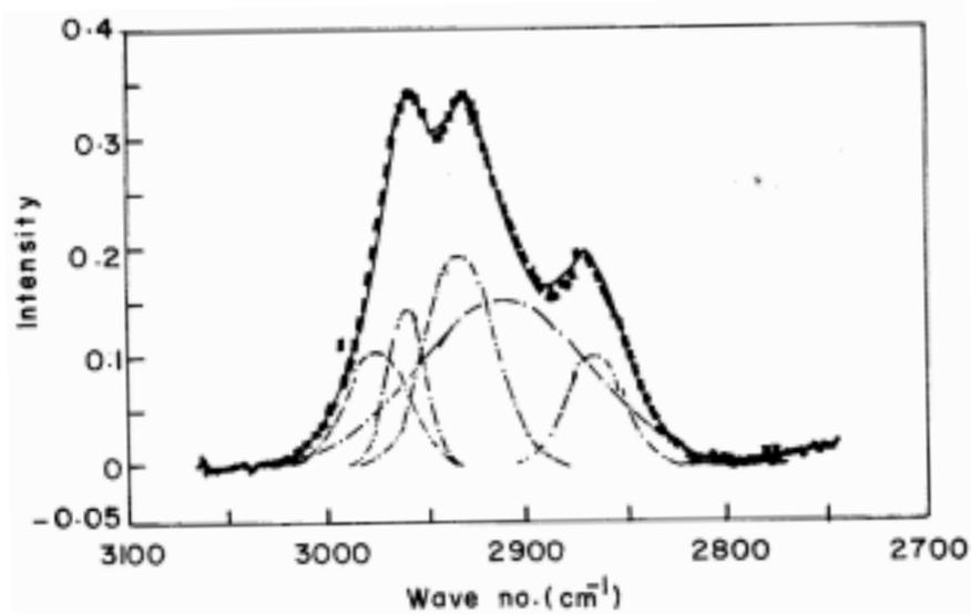
**Figure 1.** FTIR reflectance spectra (DLC on s.s.).
