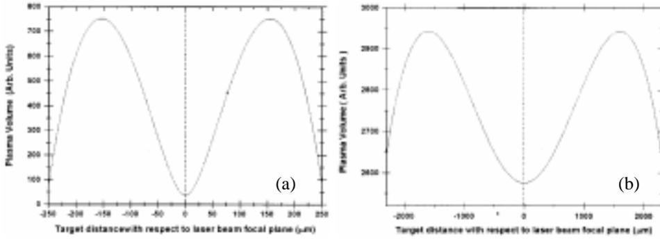
**Figure 4.** The X-ray flux that is directly proportional to the focal spot radius  $r_{th}^2$  is plotted against the target position with respect to the best laser beam focal plane. Negative values on x-axis imply that the point of laser focus is in front of the target surface, while positive values imply that the point of laser focus is behind the target surface. Results are for copper target (a) for Tallents data points and (b) for our own experimental parameters.
