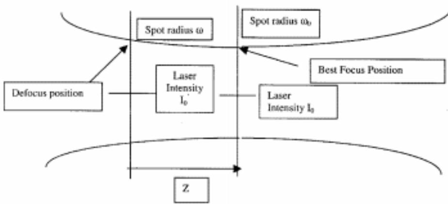
**Figure 3.** Representation of a Gaussian beam at the focal plane of a long focal length lens system.
