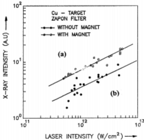
**Figure 3.** Variation of x-ray emission with laser intensity.
