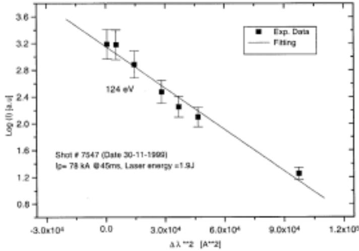
Figure 6. Electron temperature measurement of a typical plasma shot.
