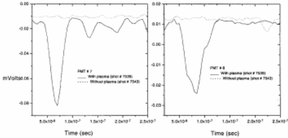
Figure 5. Example for the comparison of signals with and without plasma.
