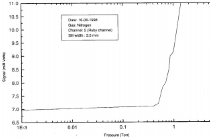
Figure 3. Rayleigh scattering for different gas pressure.
