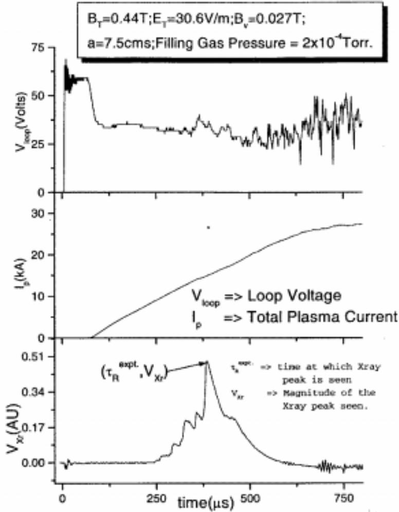
Figure 3. Typical plasma discharge in the SINP tokamak.
