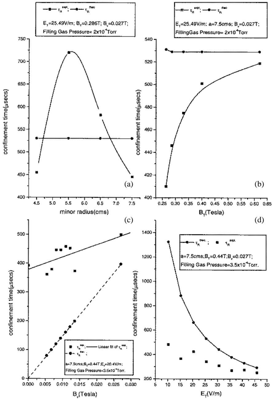
**Figure 4.** Comparison of theoretical and experimental results: (a) on variation of minor radius; (b) on variation of toroidal magnetic field; (c) on variation of vertical magnetic field and (d) on variation of applied electric field.
