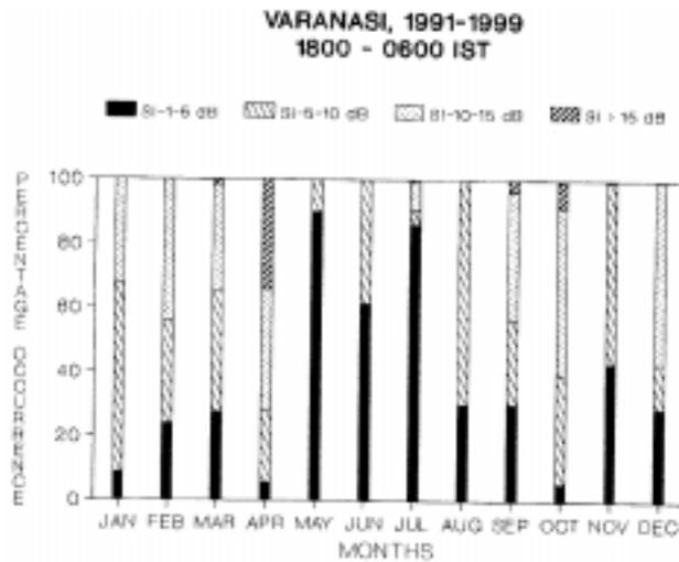
**Figure 4.** The occurrence of 15 minute fade depth indices of scintillation (in dB) for night time periods during 1991–1999.
