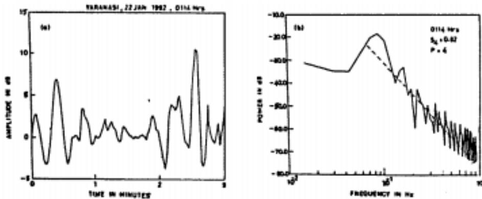
**Figure 5.** A typical example of (a) amplitude scintillation recorded at Varanasi on 22nd January 1992 at 0114 IST and their corresponding (b) power spectra.
