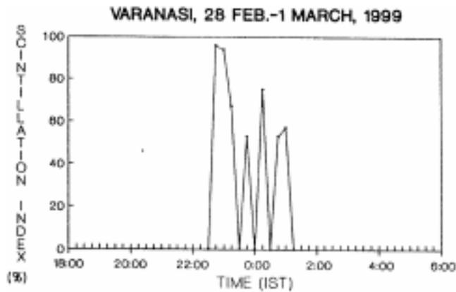
**Figure 3.** One typical example of the nocturnal variation of scintillation index (%) observed at Varanasi on 28th February–1st March 1999.
