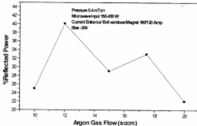
**Figure 5.** Plot of argon gas flow rate versus reflected power in the microwave power input range of 150–450 W with probe bias –30 volts at the current of window/exit magnets 180/120 amp respectively, at pressure 0.4 mTorr.
