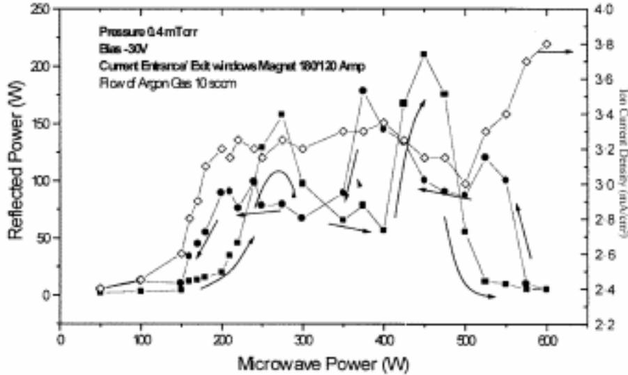
**Figure 2.** Plot of microwave input power versus reflected power and ion current density at pressure 0.4 mTorr, bias –30 volts of argon flow of 10 sccm at the current of window/exit magnets 180/120 amp respectively. Variation is from minimum to maximum and vice versa also.
