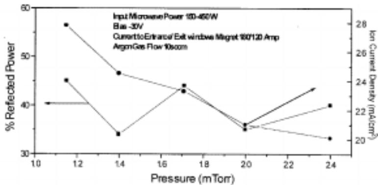
**Figure 3.** Plot of pressure versus reflected power and ion current density in the microwave power input range of 150–450 W, bias –30 volts of argon flow of 10 sccm at the current of window/exit magnets 180/120 amp respectively.
