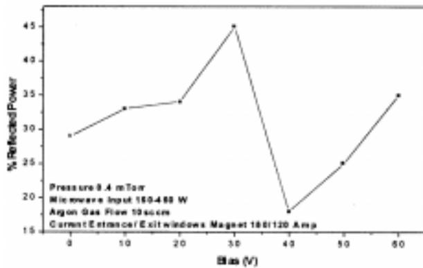
**Figure 4.** Plot of bias versus reflected power in the microwave power input range of 150–450 W of argon flow of 10 sccm at the current of window/exit magnets 180/120 amp respectively, at pressure 0.4 mTorr.
