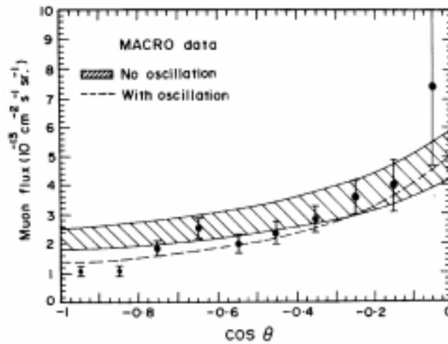
**Figure 5b.** Zenith angle distribution of up-going muons from MACRO. The solid curve with shaded region shows the expectation from no oscillation hypothesis. The dashed line shows the prediction with oscillation hypothesis using  $\Delta m^2 = 2.5 \times 10^{-3} \text{ eV}^2$  and  $\sin^2 2\theta = 1$ .
