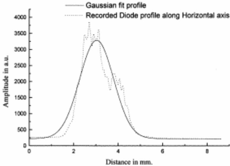
**Figure 6.** A typical magnified diode-laser profile along horizontal axis with a Gaussian fit.
