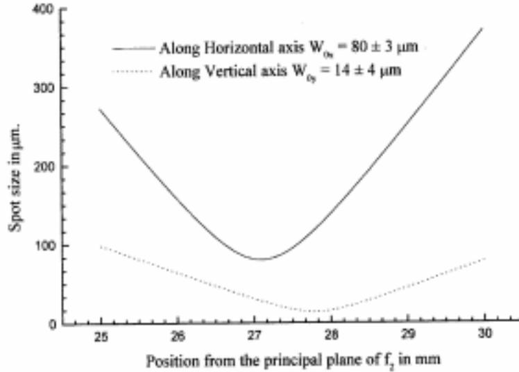
**Figure 8.** Variation of the computed waist size of the diode-laser beam with distance from the principal plane of the focusing lens.
