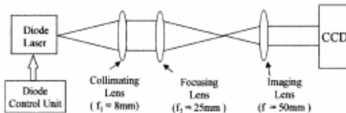
**Figure 5.** Experimental setup for recording the diode laser beam profiles.
