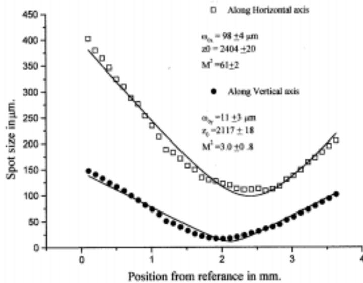
**Figure 7.** Measured variation of spot size with distance from a reference plane. The entrance plane of the imaging lens was the reference plane. Solid line corresponds to least square fit of eq. (7). The values of  $M^2$  and  $W_0$  are for Gaussian fit method. To obtain corresponding second-moment method values the appropriate scale factor has to be used.
