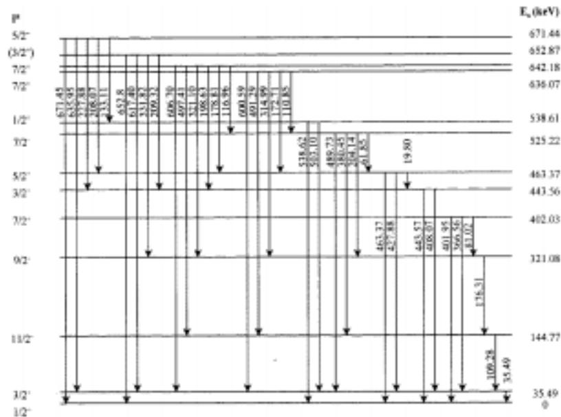
**Figure 3.** Level scheme of  $^{125}\text{Te}$  deduced from the gamma and conversion electron spectra measurements following  $^{125}\text{Sb}$  beta decay. The labelling on the left is that of the level spin and its parity, while that on the right is level energy (in keV) deduced from the transition energies listed in table 2 and the energy sum rule at each level.
