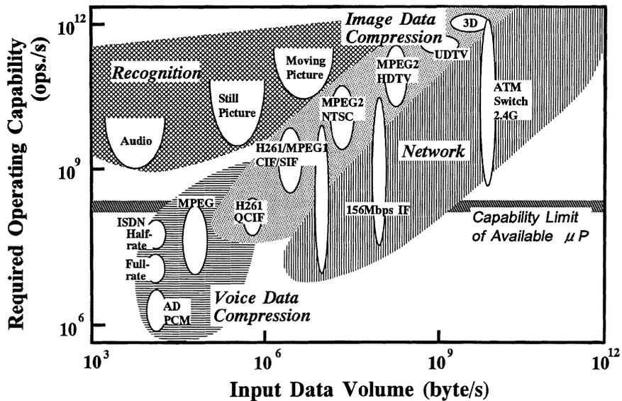
Figure 2. Operating capability of electronic systems in the multimedia digital network era (NTT).
