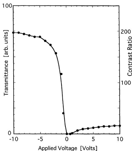
**Figure 4.** An example of the T-V characteristic curve of the PS-FLCD cell.
