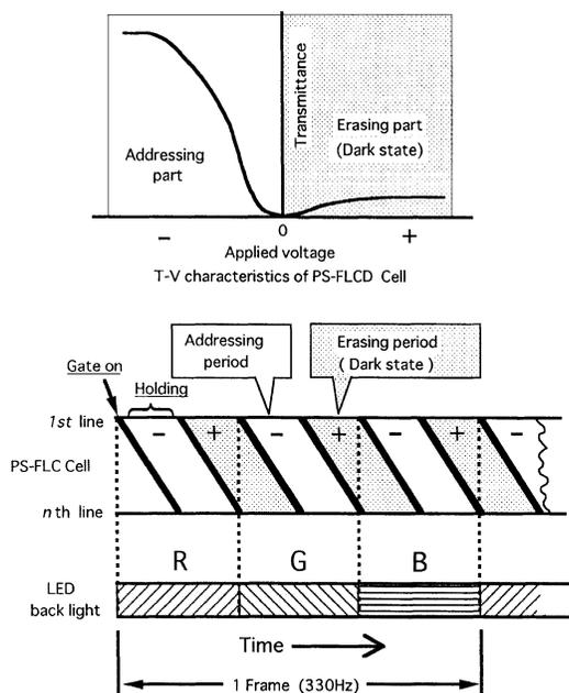
**Figure 6.** The actual timing chart of the FSC-LCD using PS-FLCD.
