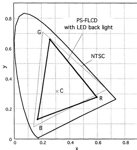
**Figure 9.** Color gamut and the white point of our FSC-LCD system on the 1931  $x$ - $y$  color coordinates.
