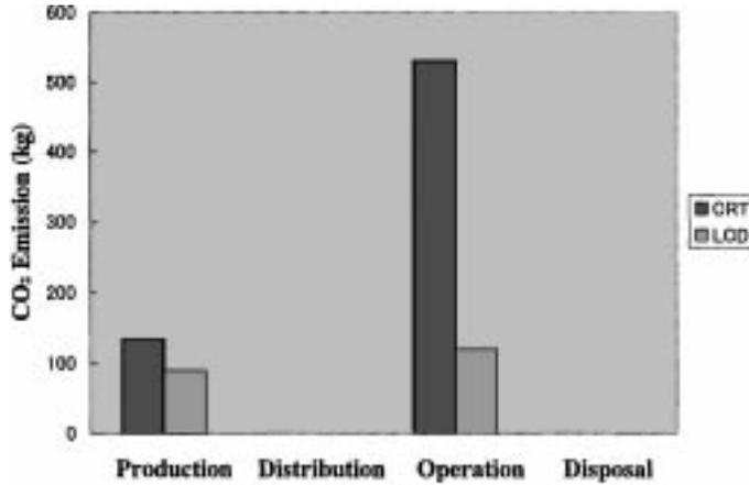
Figure 1. A comparison of the energy consumption expressed by the equivalent CO<sub>2</sub> exhaustion for computers with CRT and LCD (NEC).
