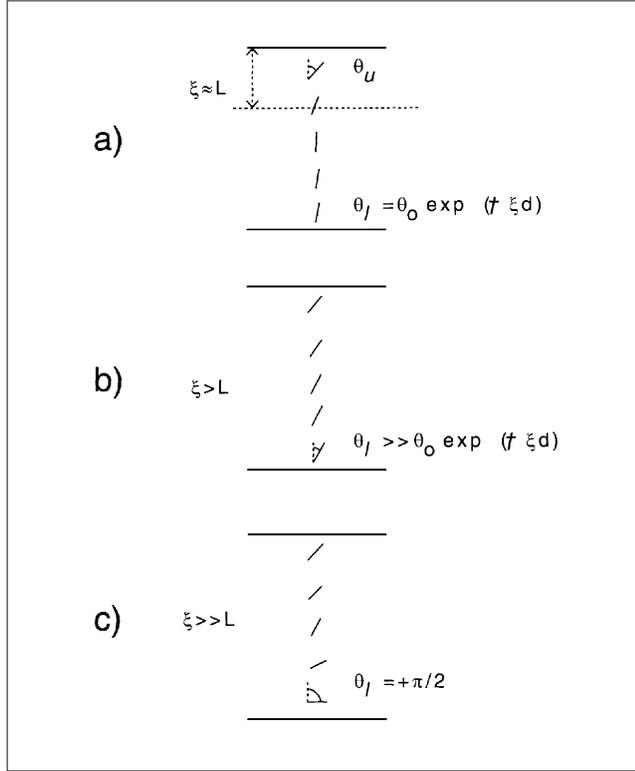
**Figure 5.** Elastic control of the bifurcation. (a)  $E > E_c$ . A small tilt remains on the lower plate, due to the elastic coupling with the upper plate. (b) At the bifurcation this small tilt is sufficient to lift the degeneracy. (c) The surface relaxation amplifies the initial tilt and leads to the  $U$ -state.
