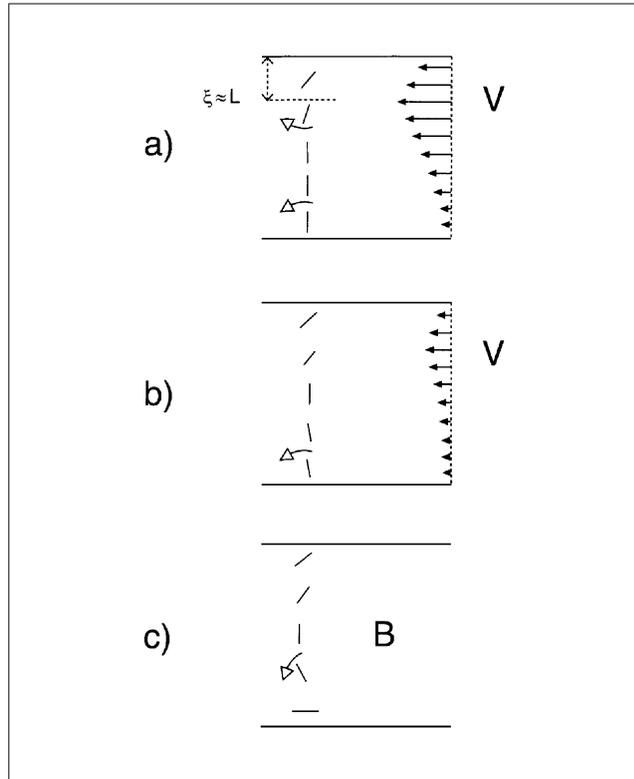
**Figure 6.** Dynamic control of the bifurcation. The field is switched off rapidly. (a) A surface flow  $v$  is created at the upper plate by the rapid director rotation. It diffuses to the lower plate almost instantaneously. (b) The hydrodynamic torque, transmitted to the lower plate director, rotates it to the opposite side from figure 5. The cell goes to state  $B$  (figure 4c, left) and  $T$ .
