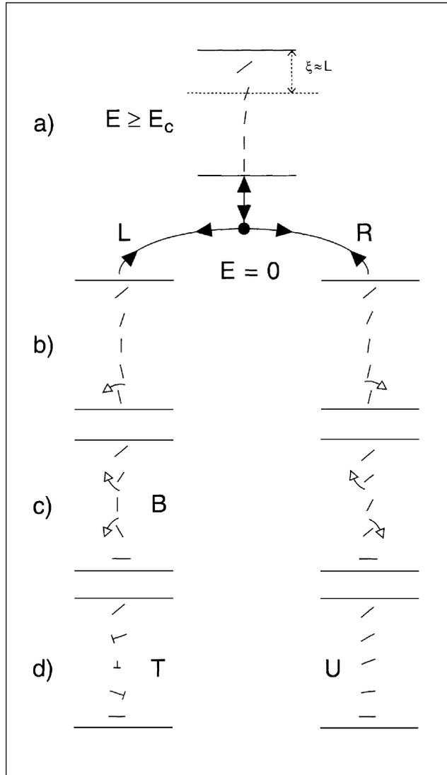
**Figure 4.** Switching by surface anchoring breaking. (a)  $E > E_c$ . Lower surface anchoring is broken. The initial state is forgotten. (b)  $E = 0$ . Relaxation towards  $U$  or  $T$ . (c) After the surface relaxation time ( $\sim 1 \mu\text{s}$ ) the anchoring is 'healed'. The final texture is topologically blocked. Half-turn of bend-splay  $B$  appears. (d)  $B$  transforms into  $T$ , topologically equivalent.
