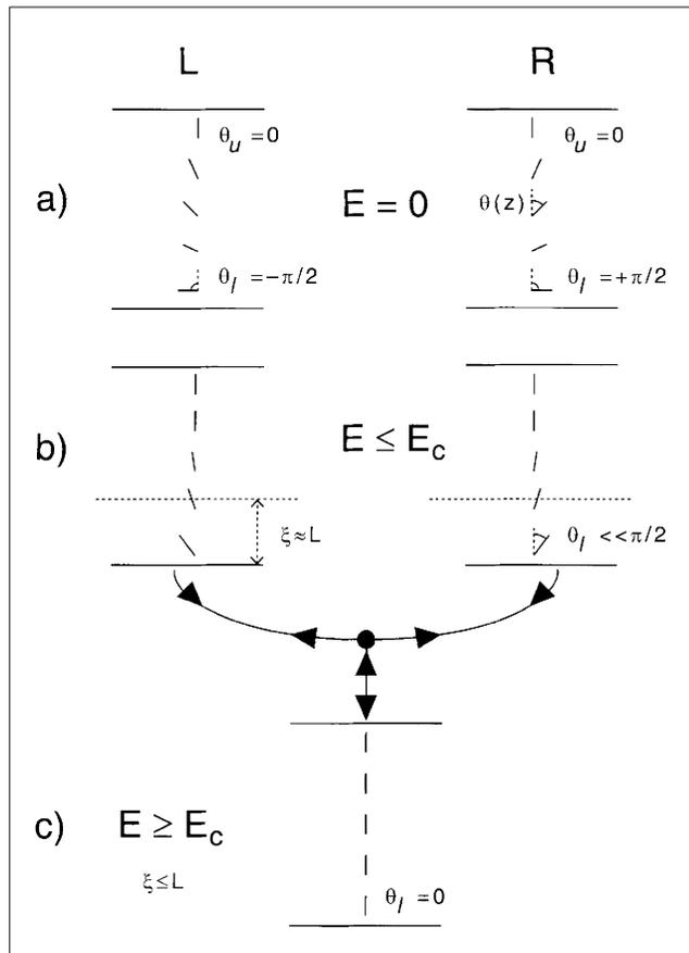
**Figure 1.** Breaking of the anchoring in a hybrid nematic cell. Left (L) and Right (R) columns present the two degenerate textures. (a)  $E = 0$ . Uniform distortion in the bulk. (b)  $E < E_c$ . Distortion near the planar plate. Surface director tilted from the easy axis. (c)  $E > E_c$ . The lower plate anchoring is broken, the sample is homeotropic.
