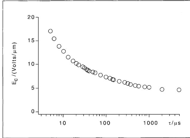
**Figure 7.** Dynamic anchoring breaking threshold for SiO aligned 5CB.
