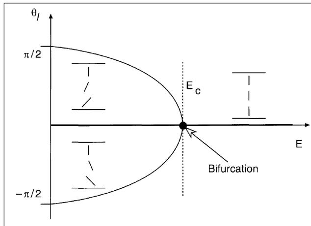
**Figure 2.** Anchoring-breaking transition under an electric field. The two symmetric branches at  $E < E_c$  join at the bifurcation point, for  $\xi_c = L$ .
