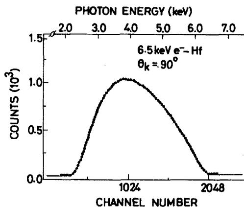
**Figure 1.** A typical bremsstrahlung X-ray photon energy spectrum produced in 6.5 keV  $e^-$ -Hf collisions. Photons are detected at  $\theta_k = 90^\circ$  with respect to the incident electron beam direction.
