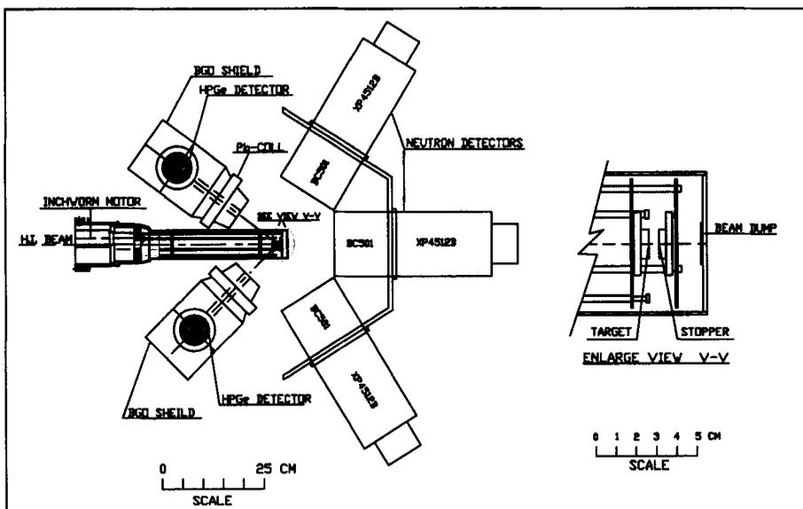
Figure 1. Schematic diagram (top view) of the recoil distance set-up neutron array and CS-HPGe detectors.
