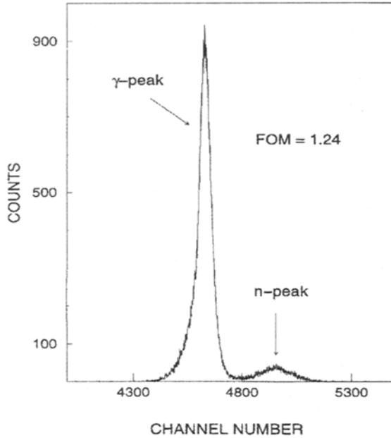
**Figure 2.** A typical spectrum from one of the neutron detectors showing the neutron and  $\gamma$  peaks after  $n - \gamma$  discrimination. The figure of merit  $FOM = 1.24$  was obtained from this detector.
