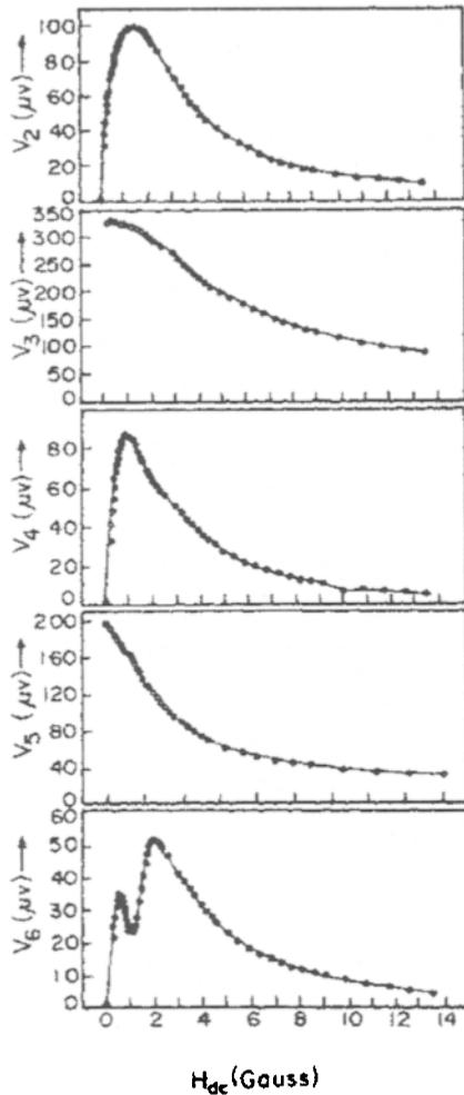
**Figure 6.** Variation of amplitude of harmonics  $V_2$ ,  $V_3$ ,  $V_4$ ,  $V_5$  and  $V_6$  for film A with  $H_{dc}$  [ $H_{ac} = 4.3\text{G}$ ,  $f_{ac} = 10\text{ kHz}$ ,  $T = 77\text{ K}$ ].
