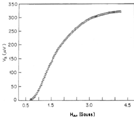
**Figure 4.** Variation of amplitude of the third harmonic ( $V_3$ ) with  $H_{ac}$  at 77K ( $H_{dc} = 0$ ) for film A.
