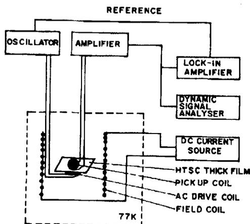
**Figure 1.** Schematic diagram of the experimental set-up used for observing the harmonic generation effect in a high- $T_c$  superconducting thick film.
