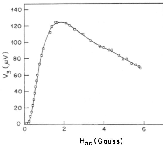
**Figure 5.** Variation of  $V_3$  with  $H_{ac}$  [ $f_{ac} = 10$  kHz] at 77K for film B.
