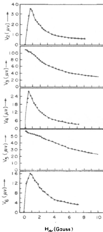
**Figure 7.** Variation of amplitude of harmonics  $V_2$ ,  $V_3$ ,  $V_4$ ,  $V_5$  and  $V_6$  for film B with  $H_{dc}$  [ $H_{ac} = 1.7G$ ,  $f_{ac} = 10$  kHz,  $T = 77K$ ].
