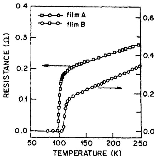
Figure 2. Resistance-temperature plot of thick films A and B.
