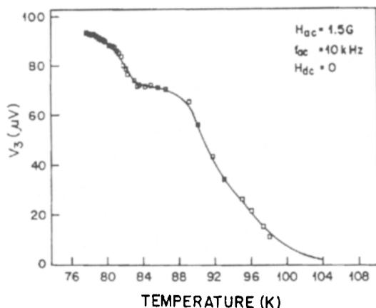
**Figure 10.** Variation of  $V_3$  with temperature for film B [ $H_{ac} = 1.5G$ ,  $H_{dc} = 0$  and  $f_{ac} = 10$  kHz].
