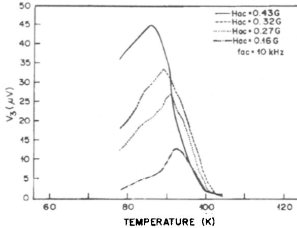
**Figure 8.** Variation of  $V_3$  with temperature at different applied ac fields for film B. [ $f_{ac} = 10$  kHz].
