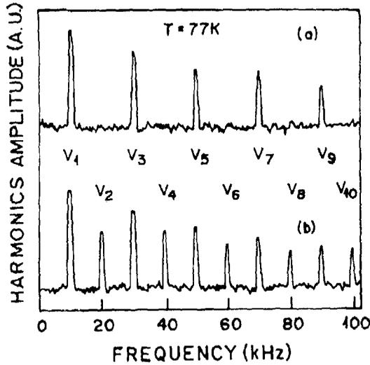
Figure 3. Frequency spectrum of the signal at pick-up coil for Bi(Pb) SrCaCuO thick film A: (a)  $H_{ac} = 4.3G$ ,  $f_{ac} = 10$  kHz,  $H_{dc} = 0$ ,  $T=77K$  (b)  $H_{ac} = 4.3$  G,  $f_{ac} = 10$  kHz,  $H_{dc} = 0$ ,  $T = 77$  K.
