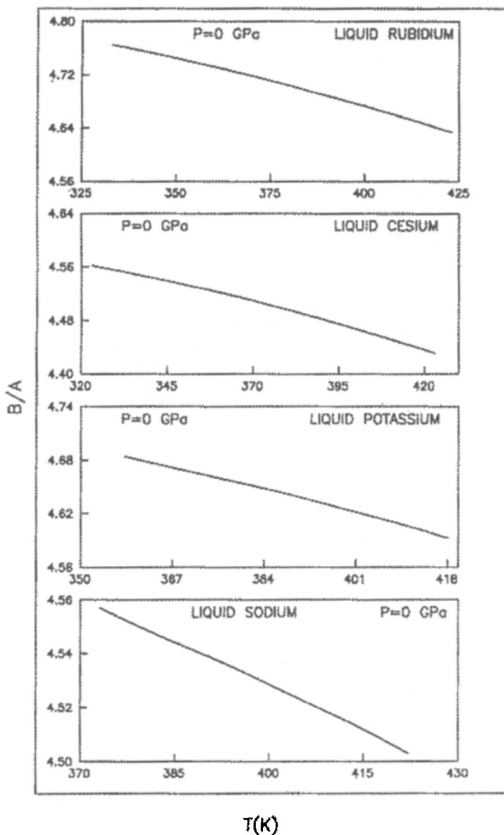
**Figure 4.** Variation of  $B/A$  as a function of temperature in case of liquid Na, K, Cs and Rb.
