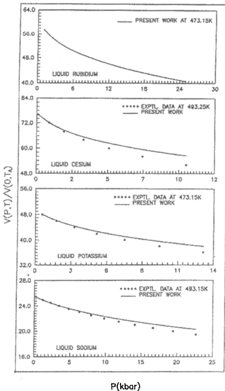
**Figure 2.** Variations  $V(P, T)/V(0, T_A)$  as a function of pressure at indicated temperature in case of liquid Na, K, Cs and Rb.
