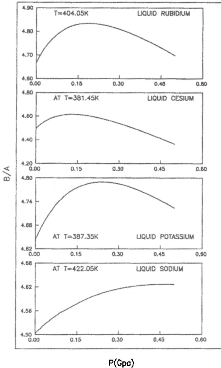
Figure 3. Variation of  $B/A$  as a function of pressure in case of liquid Na, K, Cs and Rb.
