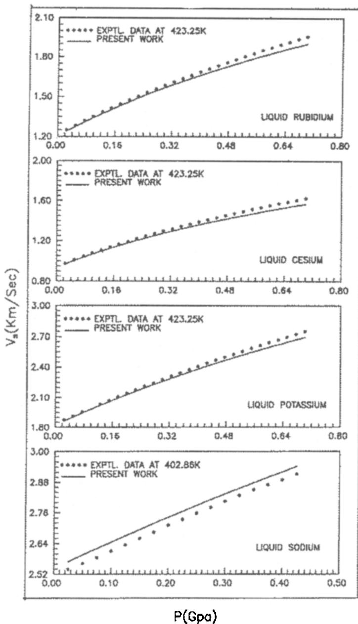
**Figure 1.** Variation of sound velocity,  $V_s$ , as a function of pressure at indicated temperature in case of liquid Na, K, Cs and Rb.
