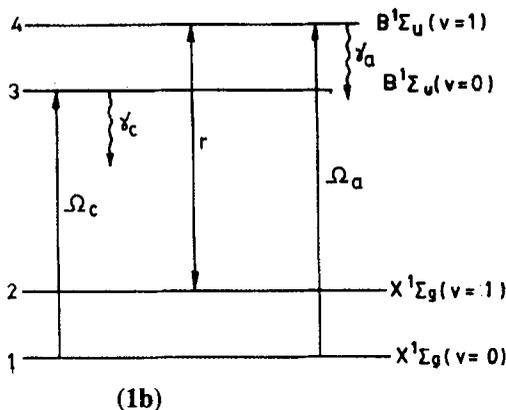
Figures 1(a) and (b). Schematic diagrams for the transition schemes considered in the  $H_2$  molecule.
