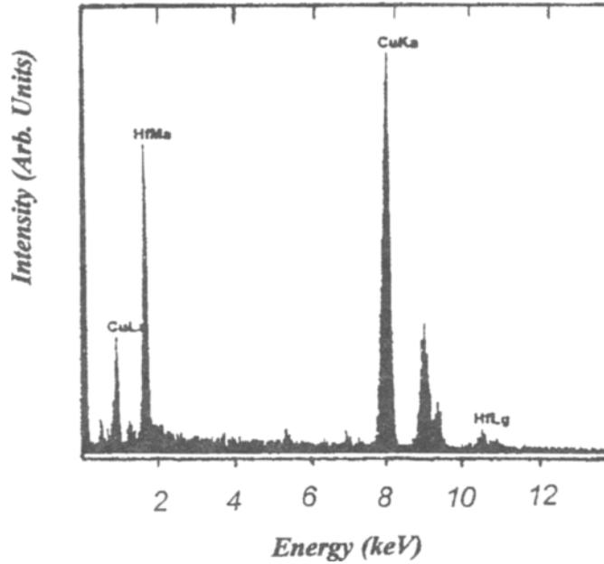
**Figure 2.** Energy dispersive x-ray analysis (EDAX) spectra showing the presence of Hf rich zones in  $\underline{\text{CuHf}}$ .
