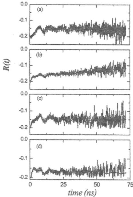
**Figure 5.** The TDPAC spectra in the room temperature helium ions implanted  $\underline{\text{CuHf}}$  sample subjected to following annealing treatments. (a) as implanted (b)  $T_a = 473$  K (c)  $T_a = 773$  K and (d)  $T_a = 873$  K.
