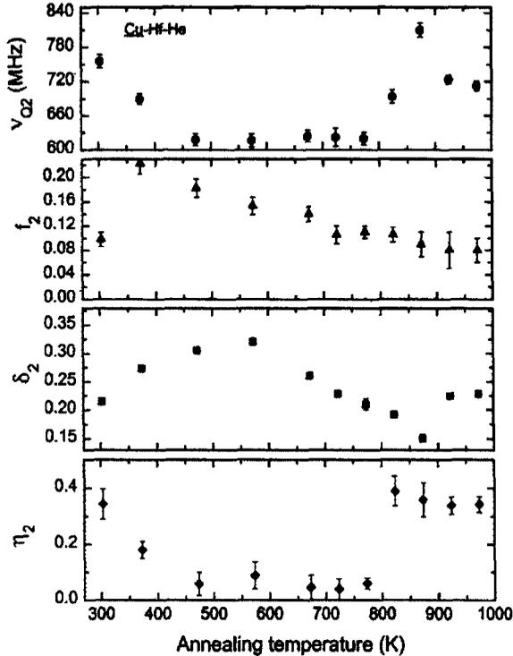
Figure 7. Variation of hyperfine interaction parameters viz.  $\nu_{Q2}$ ,  $f_2$ ,  $\eta_2$  and  $\delta_2$  with isochronal annealing temperature.
