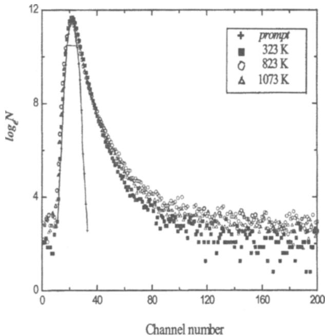
**Figure 3.** The positron decay spectra at room temperature in helium implanted  $\underline{5\text{CuHf}}$  sample subjected to annealing treatments at 323, 823 and 1073 K. Also shown in the figure is the prompt spectrum obtained with  $^{60}\text{Co}$  having a FWHM of 220 ps.
