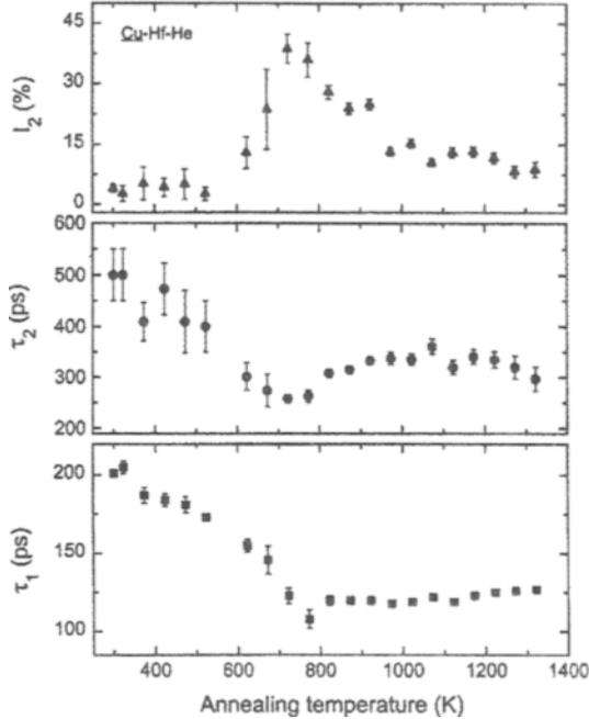
**Figure 4.** Variation of the resolved positron lifetime parameters viz.  $\tau_1$ ,  $\tau_2$  and  $I_2$  with isochronal annealing temperature.
