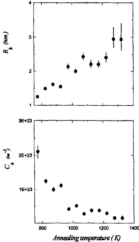
Figure 8. Variation of (a) bubble radius and (b) bubble concentration with annealing temperature in the helium implanted CuHf as deduced from the positron lifetime results.
