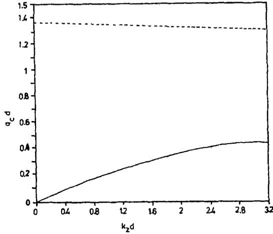
**Figure 2.** Critical  $q$ -values as a function of  $k_z d$  for coupled electron-hole plasma oscillations. The solid curve corresponds to electron plasma, whereas dash-dash curve corresponds to hole plasma oscillations.
