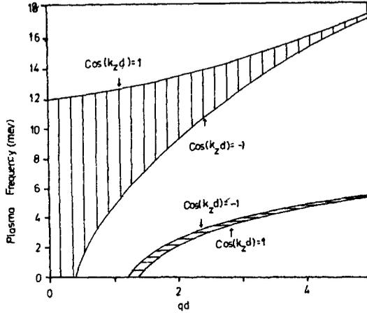
Figure 1. The coupled electron-hole plasma frequencies as a function of  $qd$ .
