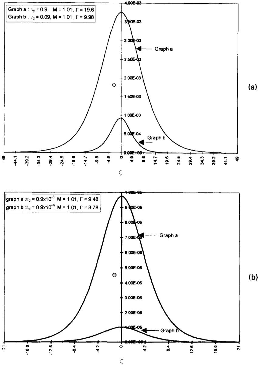
**Figure 2(a).** Soliton profile  $\Phi$  versus  $\zeta$  for  $\epsilon_d = 0.9$  and  $\epsilon_d = 0.9 \times 10^{-1}$ ;  $M = 1.01$ ,  $T_e = 1.0 \text{ eV}$ ,  $T_i = 0.1 \text{ eV}$ . **(b).** Soliton profile  $\Phi$  versus  $\zeta$  for  $\epsilon_d = 0.9 \times 10^{-3}$  and  $\epsilon_d = 0.9 \times 10^{-4}$ ;  $M = 1.01$ ,  $T_e = 1.0 \text{ eV}$ ,  $T_i = 0.1 \text{ eV}$ .
