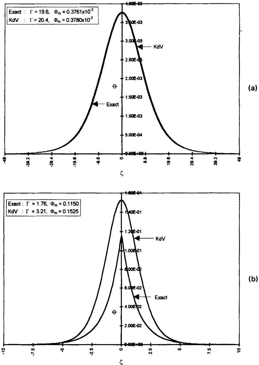
**Figure 5(a).** Soliton potential  $\Phi$  versus  $\zeta$  from exact solution and from *KdV* solution;  $\epsilon_d = 0.9, M = 1.01, T_e = 1.0 \text{ eV}, T_i = 0.1 \text{ eV}$ . **(b).** Soliton potential  $\Phi$  versus  $\zeta$  from exact solution and from *KdV* solution;  $\epsilon_d = 0.9, M = 1.60, T_e = 1.0 \text{ eV}, T_i = 0.1 \text{ eV}$ .
