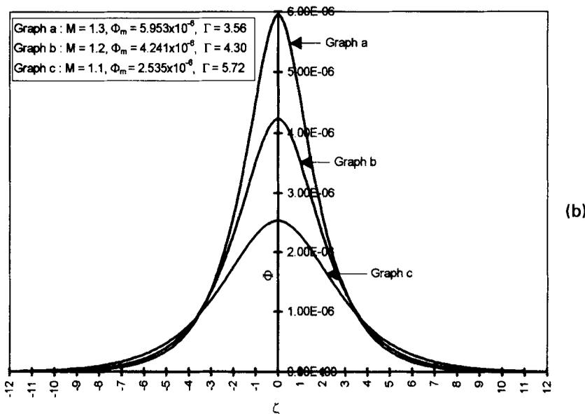
**Figure 3(a).** Soliton profile  $\Phi$  versus  $\zeta$  for  $M = 1.1, 1.2$  and  $1.3$ ;  $\epsilon_d = 0.9$ ;  $T_e = 1.0 \text{ eV}$ ,  $T_i = 0.1 \text{ eV}$ . **(b).** Soliton profile  $\Phi$  versus  $\zeta$  for  $M = 1.1, 1.2$  &  $1.3$ ;  $\epsilon_d = 0.9 \times 10^{-4}$ ;  $M = 1.01$ ,  $T_e = 1.0 \text{ eV}$ ,  $T_i = 0.1 \text{ eV}$ .
