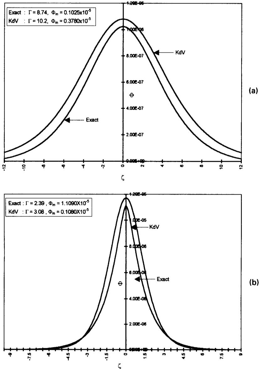
**Figure 6(a).** Soliton potential  $\Phi$  versus  $\zeta$  from exact solution and from *KdV* solution;  $\varepsilon_d = 0.9 \times 10^{-4}$ ,  $M = 1.01$ ,  $T_e = 1.0$  eV,  $T_i = 0.1$  eV. **(b).** Soliton potential  $\Phi$  versus  $\zeta$  from exact solution and from *KdV* solution;  $\varepsilon_d = 0.9 \times 10^{-4}$ ,  $M = 1.60$ ,  $T_e = 1.0$  eV,  $T_i = 0.1$  eV.
