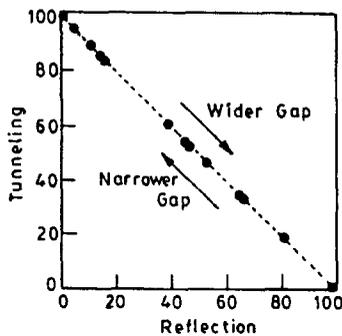
Figure 8. The relation between reflection and tunneling as the gap between the prisms is varied.
