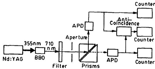
Figure 7. The anti-coincidence experiment.
