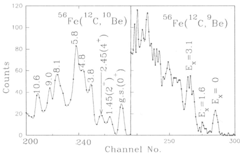
**Figure 3.** Energy spectra of  $^{10}\text{Be}$  and  $^9\text{Be}$  in  $^{56}\text{Fe}(^{12}\text{C}, X)$  reaction at  $E(^{12}\text{C}) = 60$  MeV and  $\theta_{\text{lab}} = 19^\circ$ . Excitation energies indicated in the figure are in MeV.
