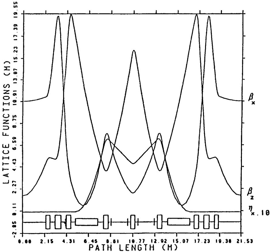
Figure 8. Lattice functions of INDUS-2.
