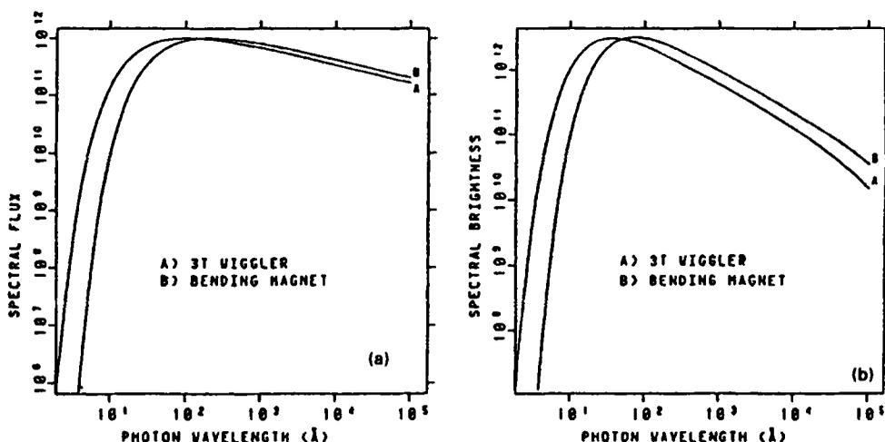
Figure 6. (a) Flux and (b) brightness versus photon wavelength for INDUS-1.
