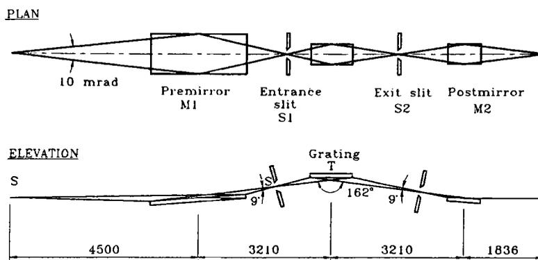
Figure 11. Optical layout of metrology beamline on INDUS-1.
