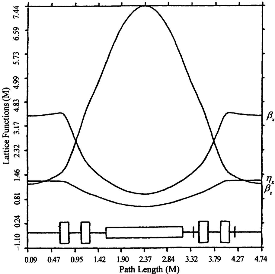
Figure 5. Lattice functions of INDUS-1.
