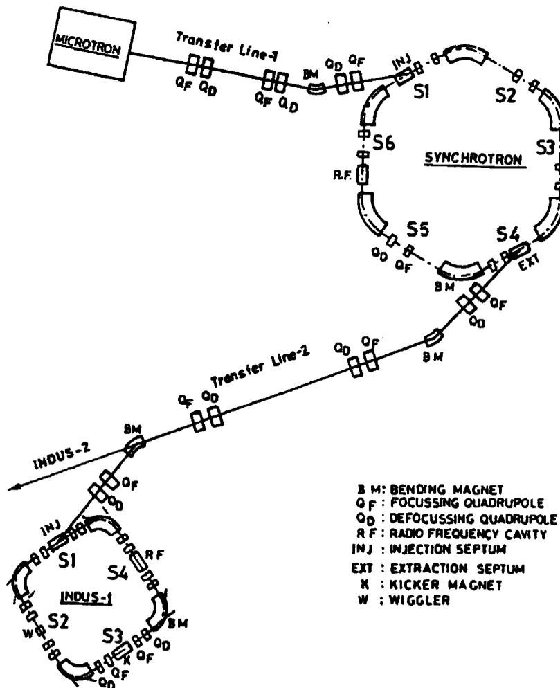
Figure 2. Schematic of injector system and INDUS-1.
