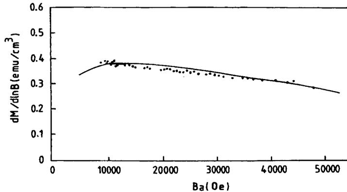
**Figure 3.** The field dependence of  $dM/d \ln B_a$  of a polycrystalline Bi(2212) sample at  $T = 55$  K. The data are taken from figure of ref. [12]. The solid line is a theoretical fit according to eq. (4) with parameters  $\lambda = 4017 \text{ \AA}$  and  $B_{c2} = 100$  T.
