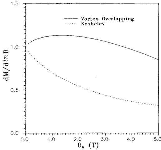
**Figure 2.**  $dM/d \ln B_a$  (in units of  $\phi_0/32\pi^2\lambda^2$ ) versus  $B_a$ . For the solid line we have taken  $B_{c2} = 10$  and for dashed line  $B_{c2} = 20$  T.
