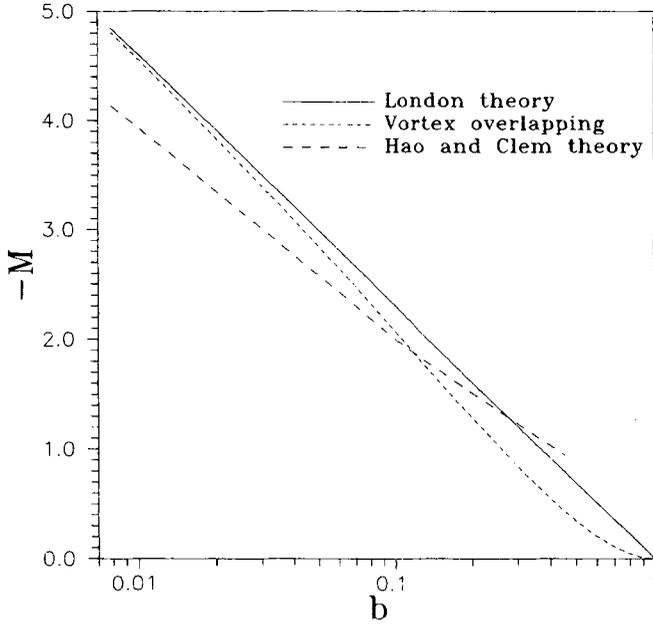
Figure 1. The magnetization (in units of  $\phi_0/32\pi^2\lambda^2$ ) vs  $b$ .
