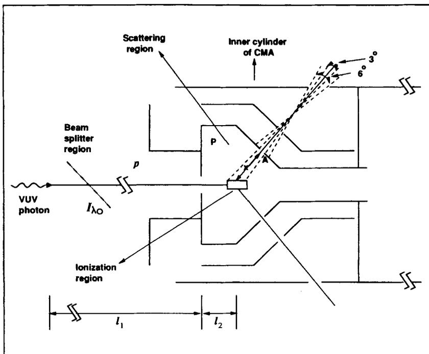
**Figure 1.** Schematic diagram showing ionization as well as the electron scattering region in the cylindrical mirror analyser of the photoelectron spectrometer.
