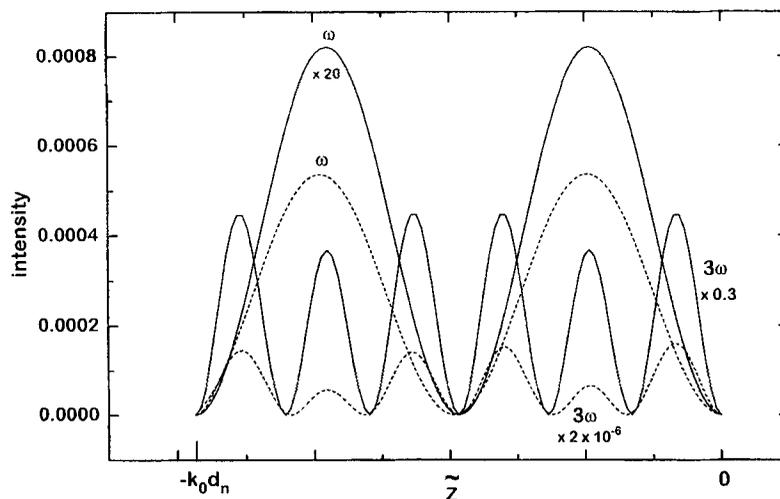
**Figure 4.** Intensity distribution along the length of the nonlinear slab of the Fabry-Perot cavity of figure 1a where electric field intensities at  $\omega$  and  $3\omega$  are plotted as a function of  $\tilde{z}$ . The solid (dashed) curve gives our (Bethune's) results. Various curves are labeled by their corresponding frequencies. Note also the different scale factors for various curves.
