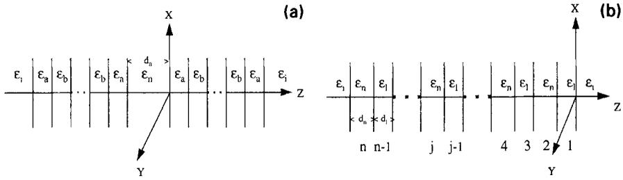
**Figure 1.** Schematic view of (a) Fabry-Perot cavity with reflection coatings with medium parameters  $\epsilon_a = 5.29$ ,  $\epsilon_b = 1.71$ ,  $\epsilon_n = 2.5408$  and  $\epsilon_i = 1$  and (b) distributed feedback structure with alternating linear and nonlinear slabs with medium parameters  $\epsilon_i = 1.71$ ,  $\epsilon_n = 2.5408$ ,  $\epsilon_i = 1$ ,  $d_l = 0.25\lambda$  and  $n = 2m = 40$ .
