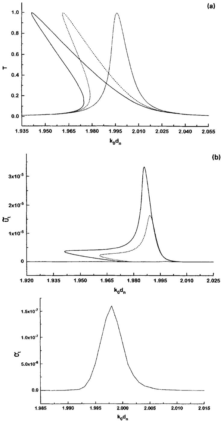
**Figure 5.** (a) Fundamental transmission  $T$  and (b) transmitted third harmonic intensity  $\tilde{U}_t$  for a Fabry–Perot cavity as functions of  $k_0 d_n$  for three different values  $U_{in}$ , namely,  $U_{in} = 3 \times 10^{-5}$  (dotted),  $3 \times 10^{-4}$  (dashed) and  $4.7 \times 10^{-4}$  (solid). Inset shows the dotted curve with a different vertical scale. Other parameters are as in figure 1a.
