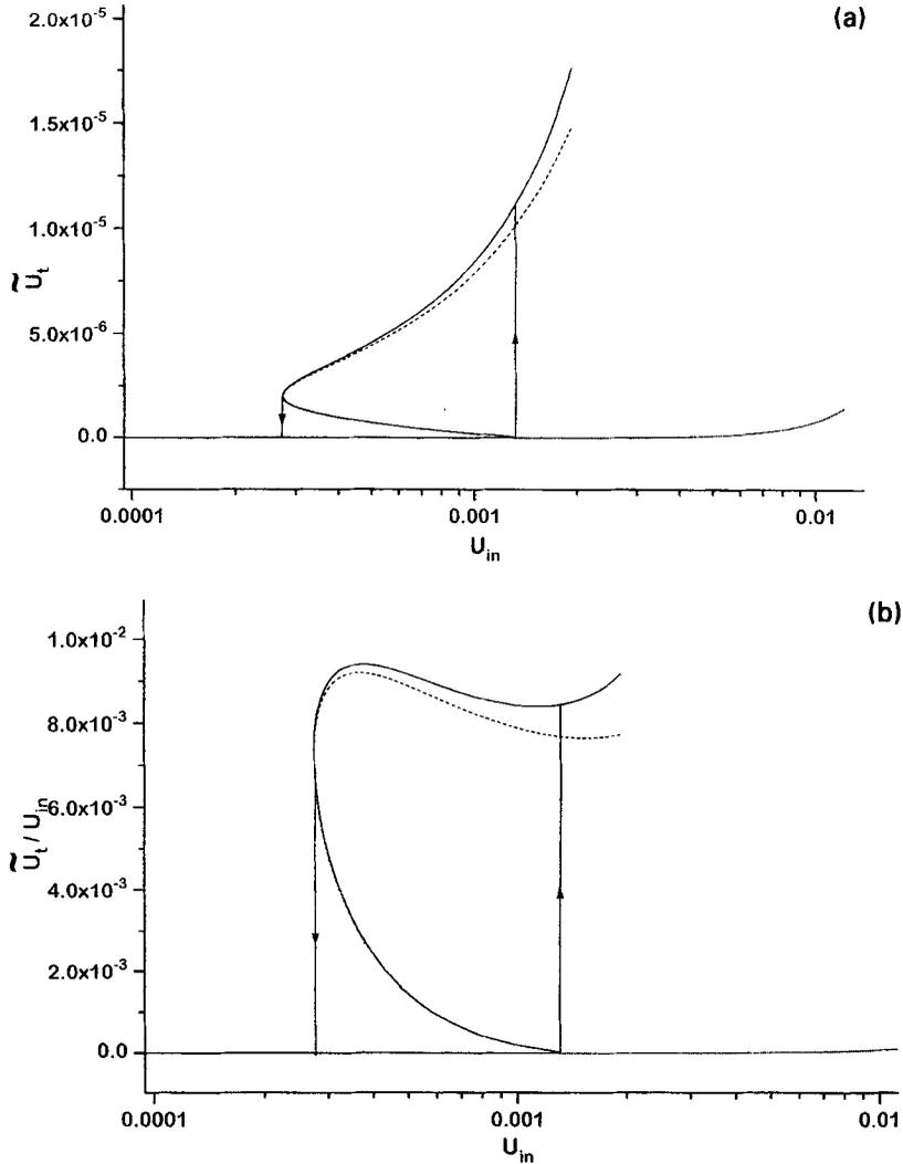
**Figure 3.** (a) Third harmonic transmitted intensity  $\tilde{U}_t$  and (b)  $\tilde{U}_t/U_{in}$  as functions of  $U_{in}$ . Solid (dotted) is with (without) self action at  $\omega$ . The dashed curve gives the result when self action at  $3\omega$  is ignored. The parameters of the cavity are as in figure 2.
