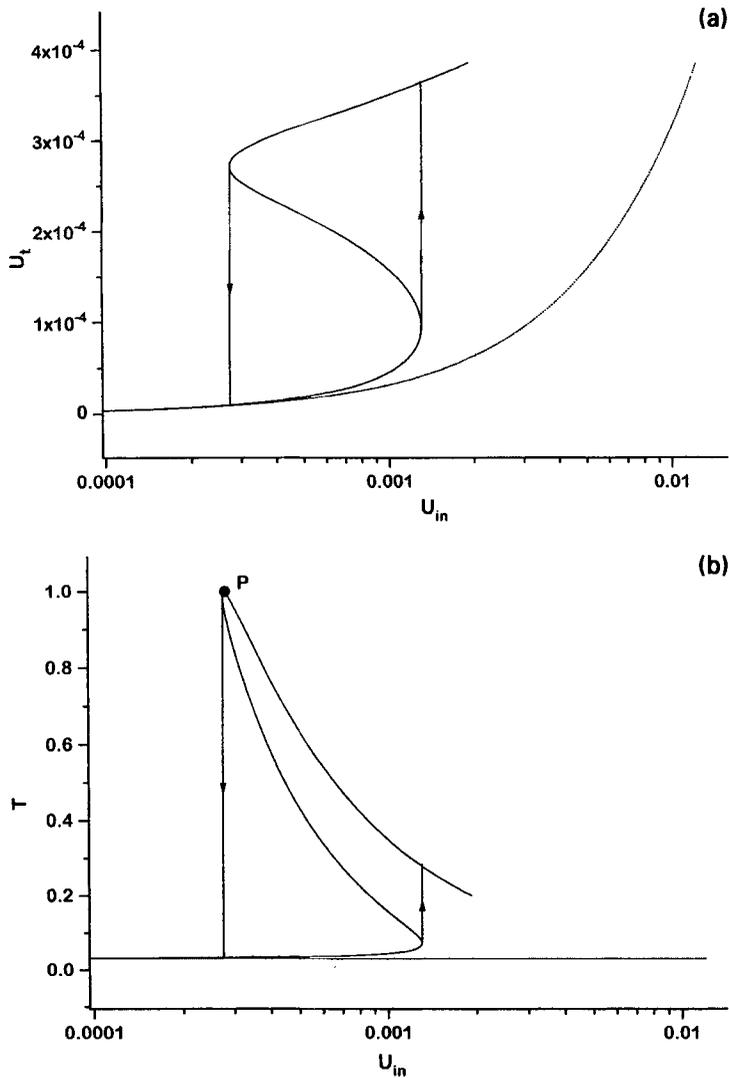
**Figure 2.** Fundamental (a) transmitted intensity  $U_t$  and (b) transmission coefficient  $T$  as functions of fundamental incident intensity  $U_{in}$  for  $k_0 d_n \sqrt{\epsilon_n} = 2(1 - \Delta)\pi$  with  $\Delta = 0.018$ . Solid (dotted) curve is with (without) self action of the fundamental. The other parameters are as in figure 1a.
