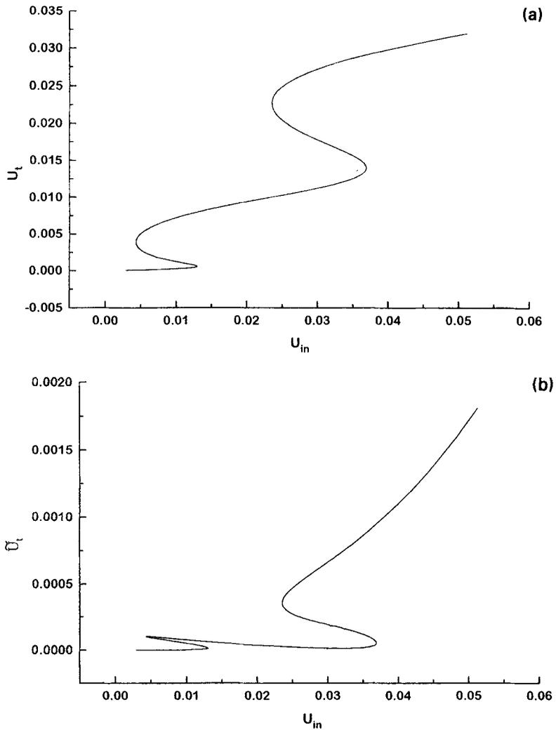
**Figure 7.** (a)  $U_t$  and (b)  $\tilde{U}_t$  as functions of  $U_{in}$  for a distributed feedback cavity for  $k_0 d_n \sqrt{\epsilon_n} = 1.391\pi$ . The other parameters are as in figure 1b.
