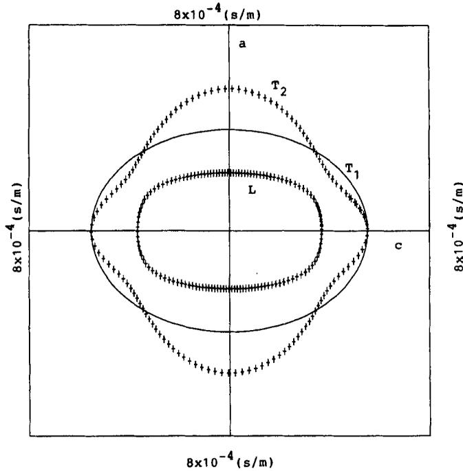
**Figure 1.** Sections of the slowness surfaces for BSCCO in the  $a$ - $c$  plane at 20 K.  $L$ ,  $T_1$  and  $T_2$  denote the quasilongitudinal, pure shear and quasishear modes respectively. Because of transverse isotropy assumed, the surfaces are concentric circles in the  $a$ - $b$  plane. Surfaces for  $a$ - $c$  and  $b$ - $c$  planes are identical.
