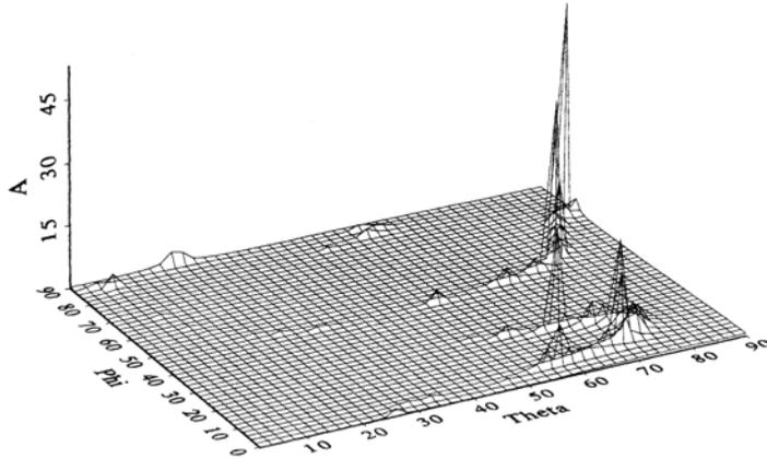
**Figure 3.** Pseudo-3D representation of the distribution of phonon intensities for the quasishear mode of BSCCO at 20 K.  $A$  is the phonon enhancement factor, with  $\theta$  (theta) and  $\phi$  (phi) designating the polar and azimuthal angles in spherical polar coordinates.
