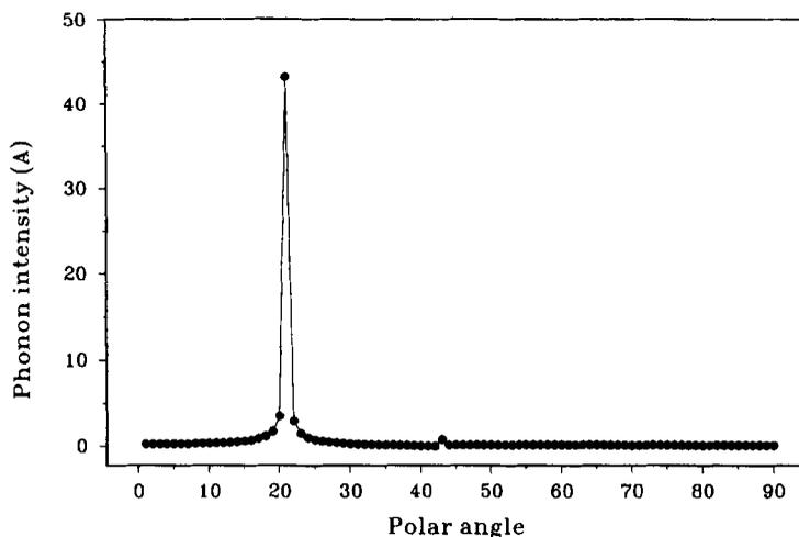
**Figure 4.** Variation of phonon intensity with the polar angle  $\theta$  for the propagation of quasishear mode in the  $a$ - $c$  plane of BSCCO at 20 K. The peak in the figure corresponds to the point at which caustics intersect the  $a$ - $c$  plane.
