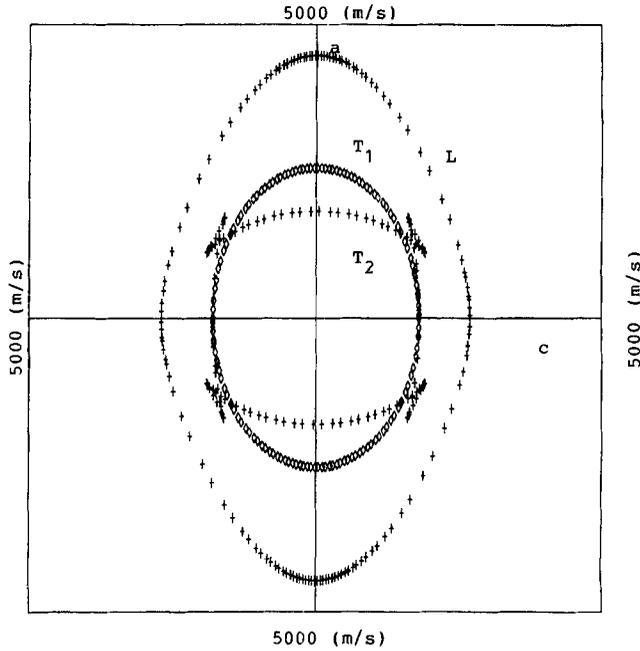
**Figure 2.** Sections of the ray velocity surfaces for BSCCO at 20 K in the *a-c* plane. L,  $T_1$  and  $T_2$  have the same meaning as in figure 1.
