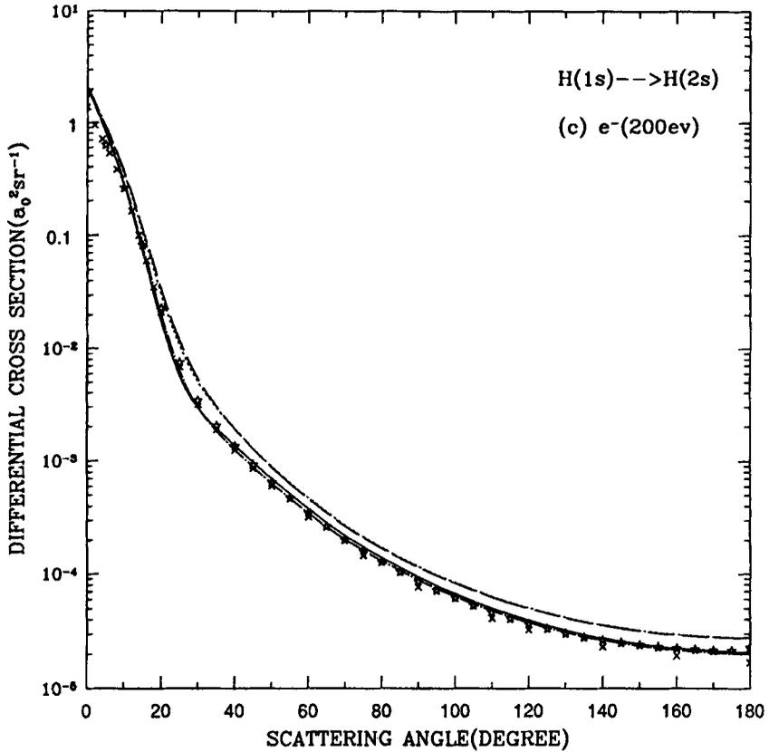
Figure 3. Differential cross sections for  $e^- + H(1s) \rightarrow e^- + H(2s)$  at 200 eV. The descriptions of the curves are the same as in figure 1.
