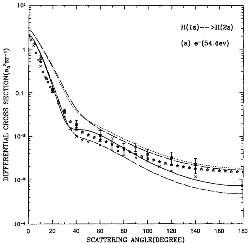
**Figure 1.** Differential cross sections for  $e^- + \text{H}(1s) \rightarrow e^- + \text{H}(2s)$  at 54.4 eV. Solid line: TCW results with exchange; dash-dot line: TCW results without exchange; dotted line: CSB2 results with exchange; dashed line: CSB2 results without exchange; stars: DWB2 results [27, 30]; crosses: 40CC results [25]; open squares with error bars: experimental results of Williams [31].
