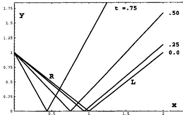
**Figure 4.** The lines  $P = 0$ ,  $R = 0$  and  $L = 0$  in the plane  $(\omega_c^2/\omega^2, \omega_p/\omega)$  corresponding to the cut-offs in a cold plasma ( $t = 0$ ) and chiroplasma for some values of  $t$ .
