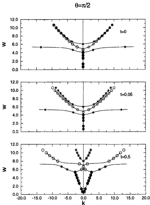
**Figure 3.** Dispersion relations for various values of the parameter  $t$  when the direction of propagation is perpendicular to the magnetic field ( $\theta = \pi/2$ ). The curves indicated by circles and stars correspond to the ordinary and extraordinary waves, respectively.
