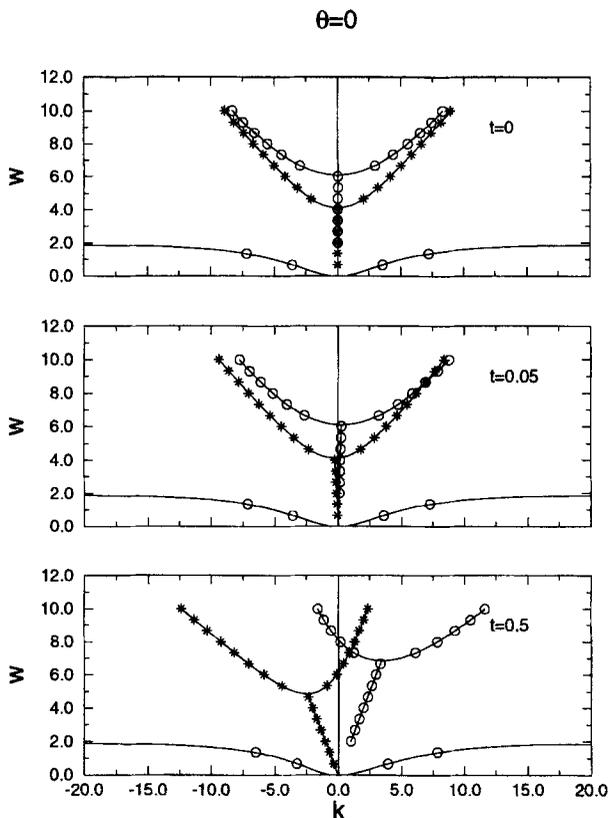
**Figure 1.** Dispersion relations for various values of the parameter  $t$  when the direction of propagation is parallel to the magnetic field ( $\theta = 0$ ). The curves indicated by circles and stars correspond to the right and left circularly polarized waves, respectively.
