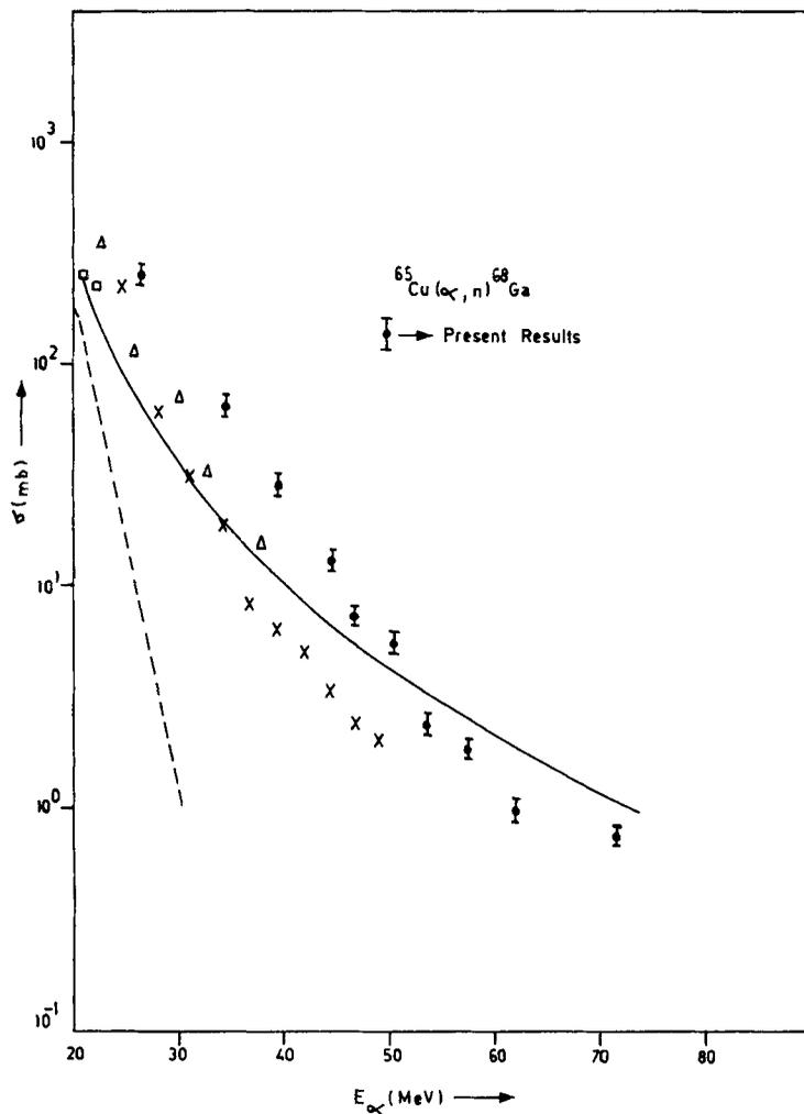
**Figure 2.** Comparison of the present and previous experimental results along with the theoretical excitation functions of  $^{65}\text{Cu}(\alpha, n)^{68}\text{Ga}$  reaction X N L Singh *et al* [25],  $\square$  Rizvi *et al* [23],  $\triangle$  Bharadwaj *et al* [24]. --- Weisskopf-Ewing estimate (W.E.), ——— hybrid model (ALICE/85/300).
