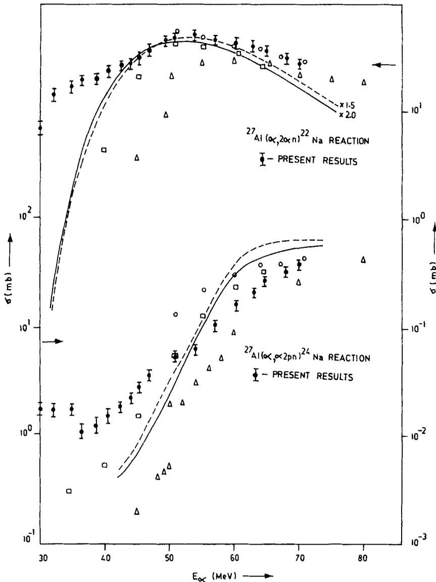
**Figure 1.** Comparison of the present and previous experimental results along with the theoretical excitation functions of (a)  $^{27}\text{Al}(\alpha, 2\alpha n)^{22}\text{Na}$ , (b)  $^{27}\text{Al}(\alpha, \alpha 2pn)^{24}\text{Na}$  reactions.  $\square$  Ismail [17],  $\circ$  Probst *et al* [16],  $\triangle$  Bowman and Blann [15], --- Weisskopf-Ewing estimate (W.E.), ——— hybrid model (ALICE/85/300).
