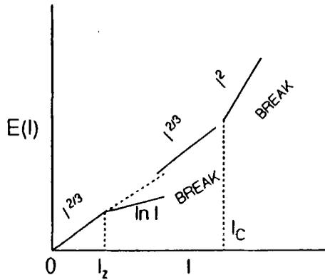
**Figure 2.** Turbulent energy spectrum.  $l_2$ , normalizing length;  $l_c$ , break due to Coriolis force [15].
