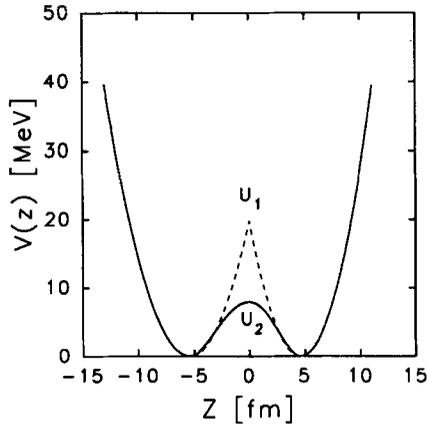
**Figure 2.** The two centre oscillator potential along the  $z$ -axis. The barrier heights without (dotted line) and with (full line) the neck potentials are  $U_1$  and  $U_2$ , respectively.
