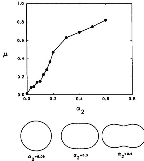
**Figure 5.** The variation of the chaos parameter  $\mu$  with deformation  $\alpha_2$  for quadrupole cavities. Dots ( $\bullet$ ) denote the calculated values and the lines are to guide the eye. Lower part shows the evolution of the cavity shape with increasing deformation.
