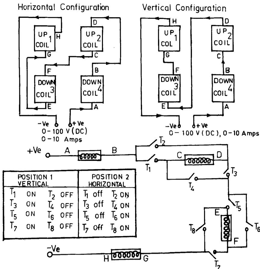
**Figure 3.** Block diagram of the electrical connections to the current carrying coils for both vertical and horizontal field configurations of the H-type electromagnet.
