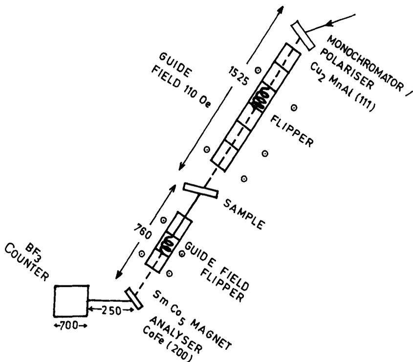
Figure 1. Schematic diagram of the polarized neutron spectrometer for neutron depolarization studies at the Dhruva reactor.
