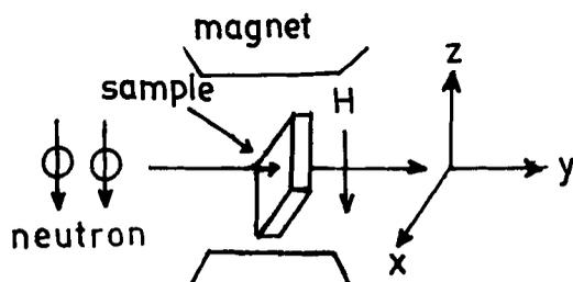
Figure 5. Schematic representation of a neutron depolarization measurement.
