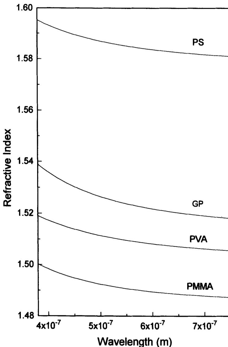
**Figure 3.** Plot of the refractive index variation with wavelength for the glass plate (GP) (average for all the plates) and the polymers PVA, PS and PMMA over the entire visible region.
