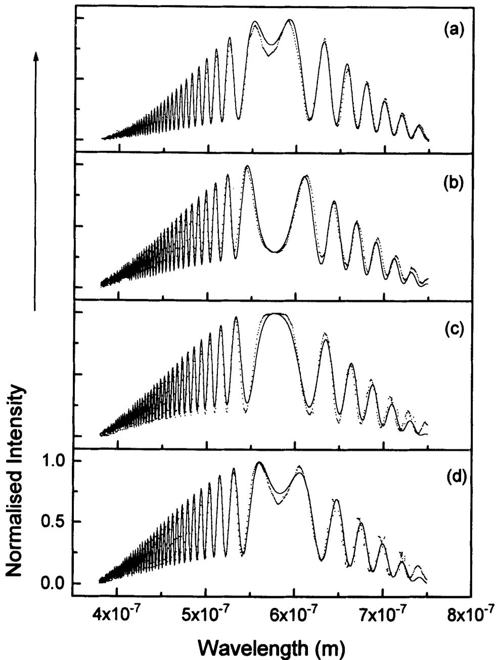
**Figure 2.** Normalized recordings of the spectral interference pattern (dotted line) and the theoretical fittings (continuous line) for (a) glass plate, (b) glass plate + PVA, (c) glass plate, (d) glass plate + PS.
