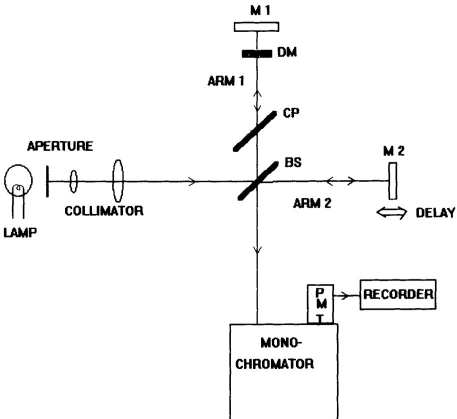
**Figure 1.** Schematic representation of the experimental set up: Michelson interferometer with the time delay between the interfering beams  $\tau > \tau_c$  ( $\tau_c$  is the correlation time of the source). BS, 50/50 beam splitter; CP, compensating plate; M1, M2, mirrors; DM, dispersive medium.
