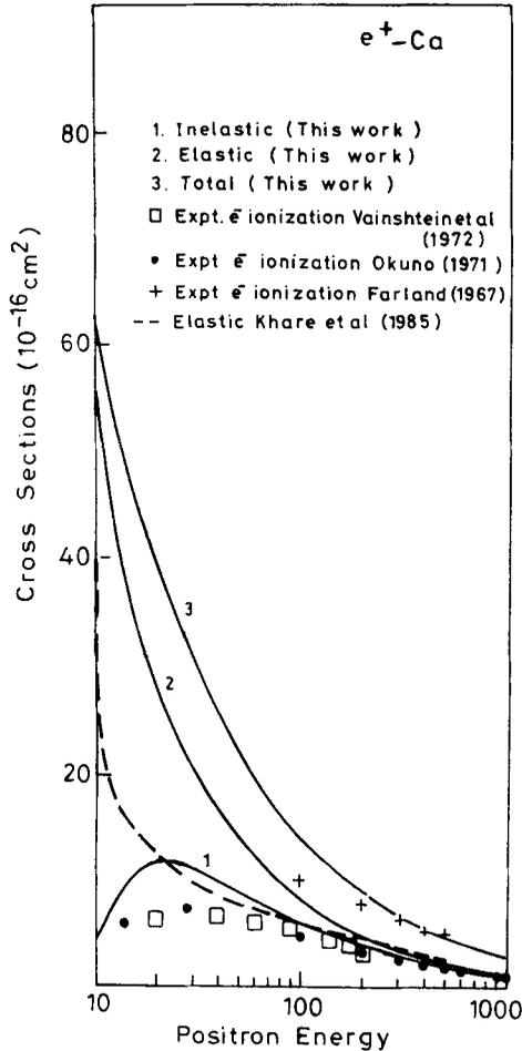
Figure 3. Cross sections for positron impact on Ca.
