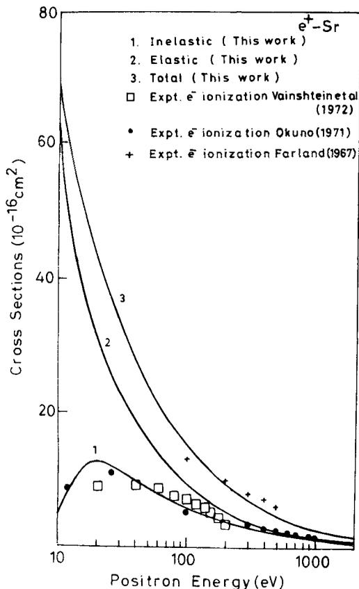
Figure 4. Cross sections for positron impact on Sr.
