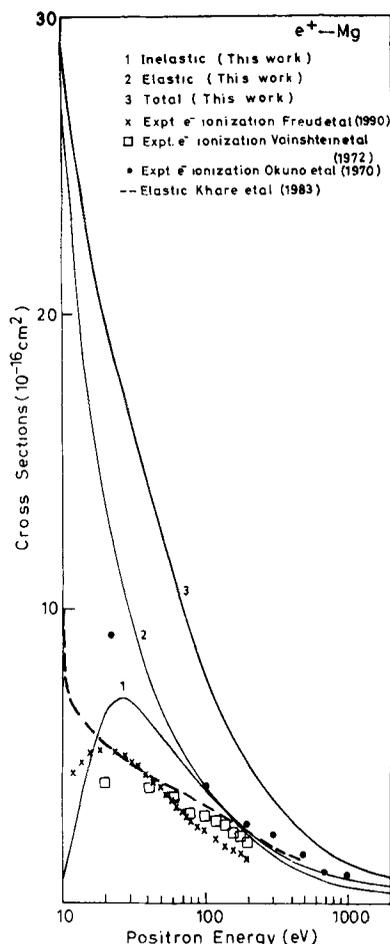
Figure 2. Cross sections for positron impact on Mg.
