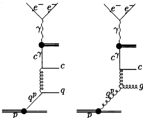
Figure 1. Excitation processes for single charm production in ep collisions
