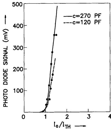
**Figure 5.** Variation of optical intensity emitted from laser diode with pumping current pulse ( $I_o/I_{Th}$ ).
