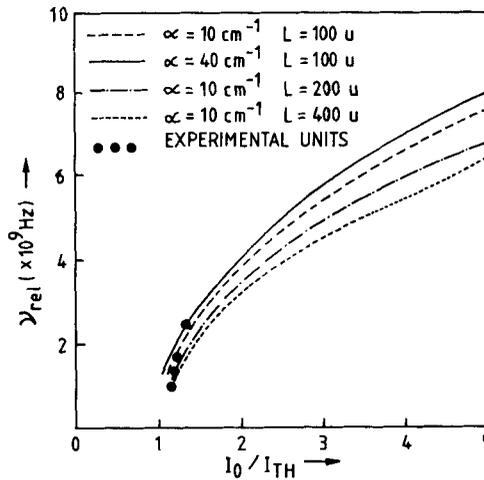
**Figure 11.** Variation of measured and calculated relaxation oscillation frequencies with pump current ( $I_0/I_{Th}$ ).
