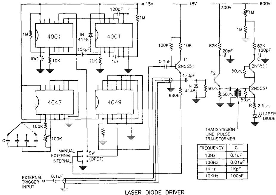
Figure 1. Circuit diagram of diode laser driver.
