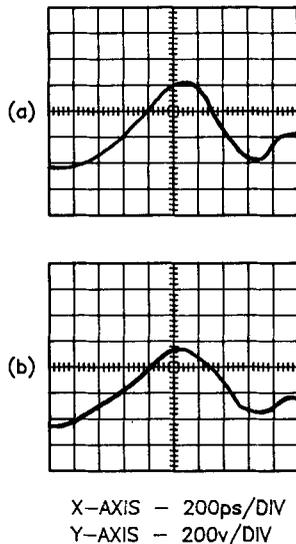
**Figure 4.** Oscilloscope of the pump pulse when series stack of nine transistors (2N5551/2N5550) were used as switching element in the driver circuit. Capacitor was charged up to (a) 2.7 kV, (b) 2.5 kV.
