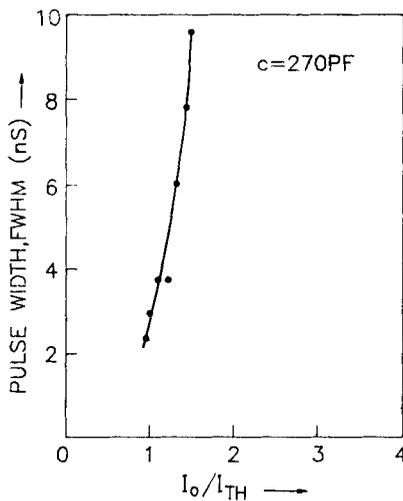
**Figure 6.** Variation of optical pulse width with the amplitude of the pump current ( $I_o/I_{Th}$ ).
