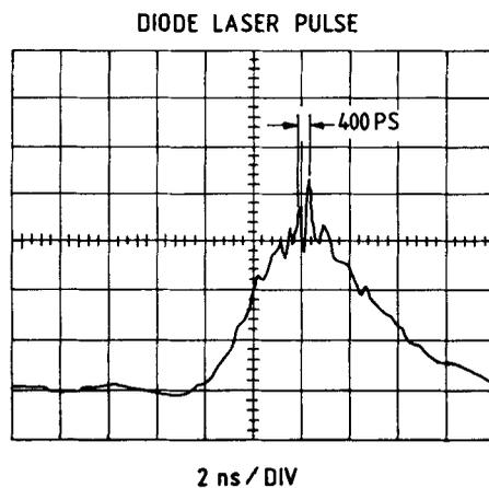
**Figure 7.** Time profile of laser diode emission (for  $I_0/I_{Th} \sim 1.32$ ) recorded using photodiode and oscilloscope (L and T Gould 100 MHz oscilloscope model 4074).
