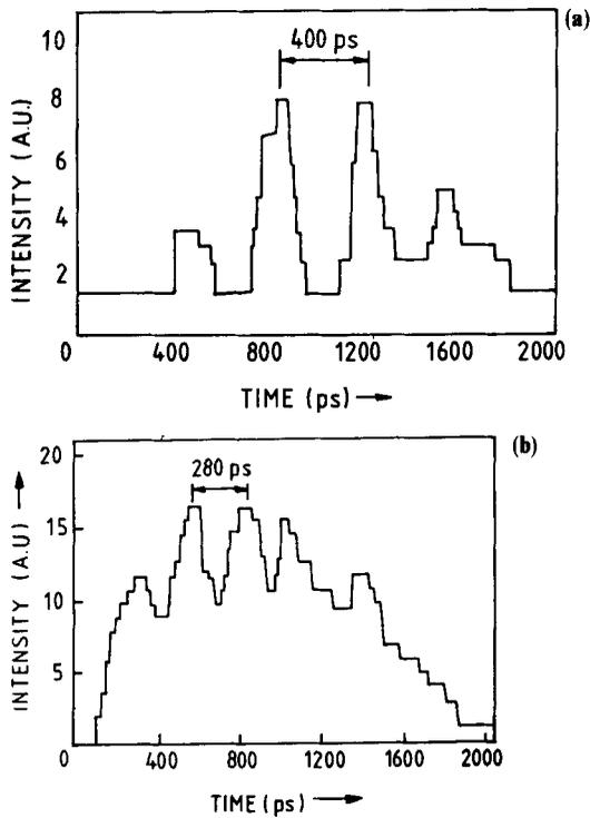
**Figure 9.** Multiple pulsation emitted from laser diode (for  $I_0/I_{Th} \sim 1.32$ ) and recorded using streak camera. (a) Laser diode I; (b) Laser diode II.
