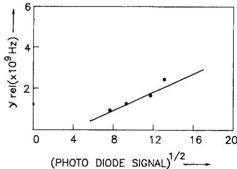
**Figure 12.** Variation of measured relaxation oscillation frequency with the square root of intensity emitted from diode laser.
