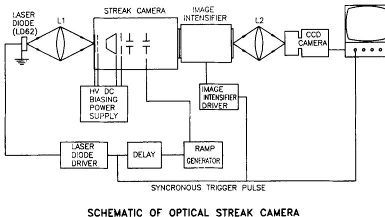
Figure 2. Schematic diagram of experimental set up.
