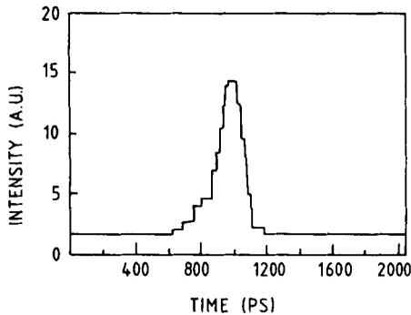
**Figure 8.** Single optical pulse from laser diode recorded using streak camera.
