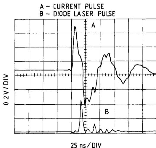
**Figure 3.** Oscilloscope trace of the electrical pump pulse when series stack of two transistors (2N5551/2N5550) were used as switching element and the optical pulse obtained from diode laser.
