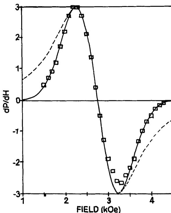
Figure 4. ESR curve of 125 K. --- Lorentzian fit. — Gaussian fit. □ expt. points.
