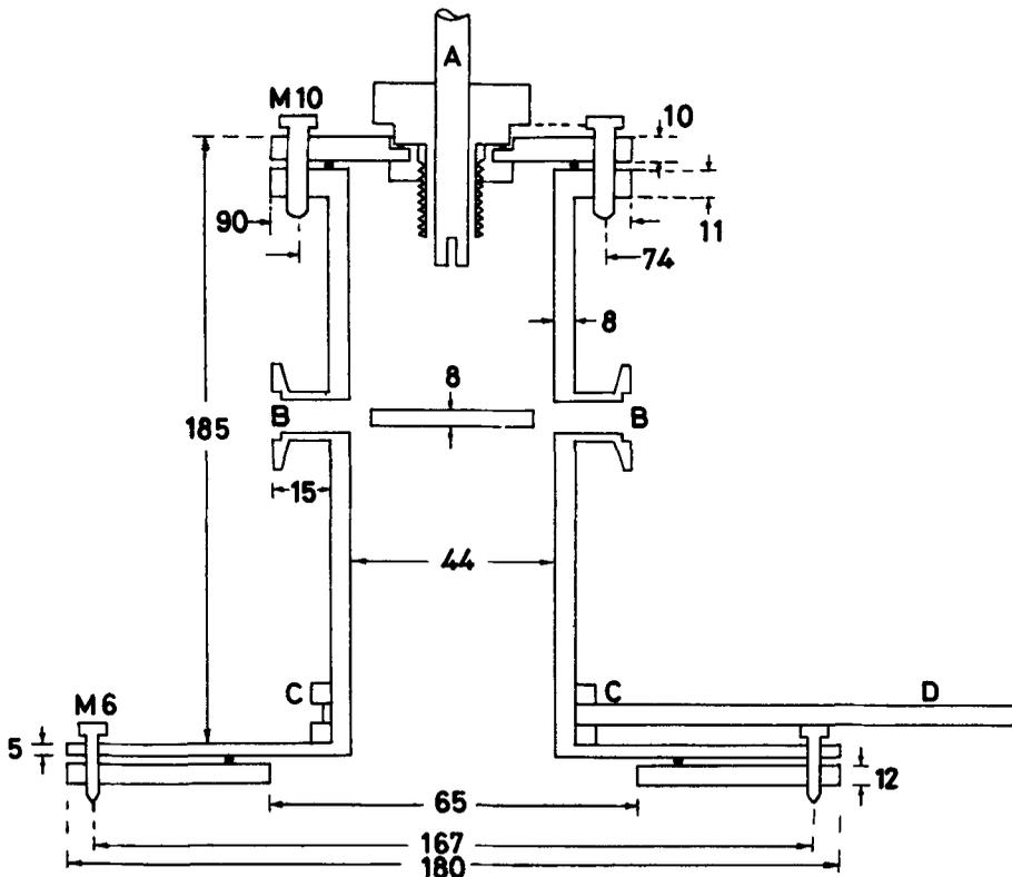
**Figure 1a.** Cross-section view of the main scattering chamber. A:  $\phi$  10 mm rotational vacuum feedthrough; B: KF 10; C: SS-collar; D: Al-rotatable platform.
