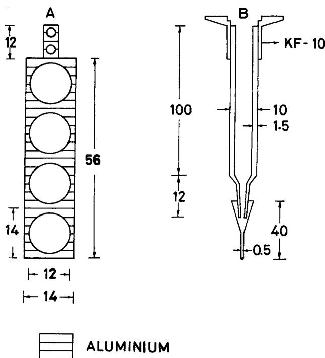
**Figure 1c.** Solid and gas target devices. A: solid target holder; B: gaseous target device.
