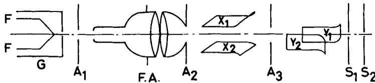
**Figure 2b.** Schematic sketch of the electron gun with different electrodes. FF: Filament; G: Grid; A<sub>1</sub>, A<sub>2</sub>, A<sub>3</sub>: Anodes; F.A.: Focussing anode; X<sub>1</sub>-X<sub>2</sub>, Y<sub>1</sub>-Y<sub>2</sub>: Deflector plates; S<sub>1</sub>, S<sub>2</sub>: Collimating slits.
