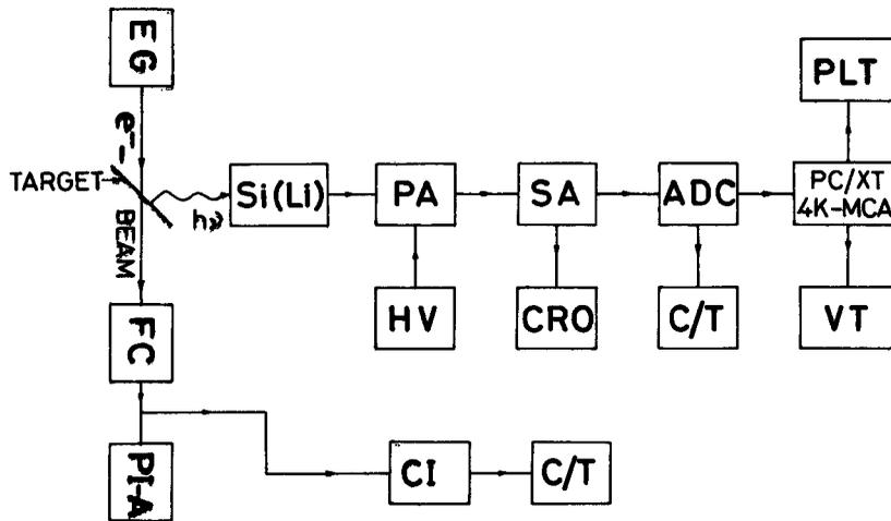
**Figure 4.** Signal processing and data acquisition system. PA: Preamplifier; SA: Spectroscopy amplifier; ADC: Analog to digital converter; HV: High voltage power supply; CRO: Cathode ray oscilloscope; C/T: Counter timer; VT: Video terminal; PLT: Plotter, CI: Current integrator; PI-A: Pico ammeter; FC: Faraday cup; EG: Electron gun.
