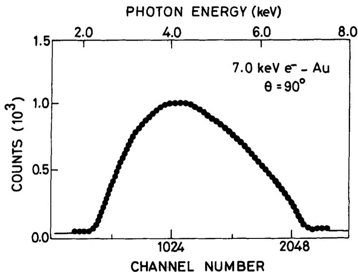
**Figure 5b.** Electron bremsstrahlung photon energy spectrum for 7.0 keV electrons on a thin Au target.
