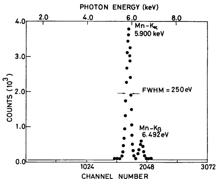
Figure 6. A typical photon energy spectrum from a  $^{55}\text{Fe}$  radioactive source.
