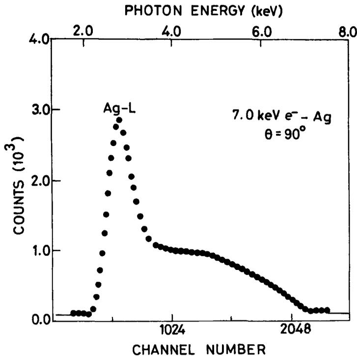
**Figure 5a.** Electron bremsstrahlung photon energy spectrum for 7.0 keV electrons on a thin Ag target.
