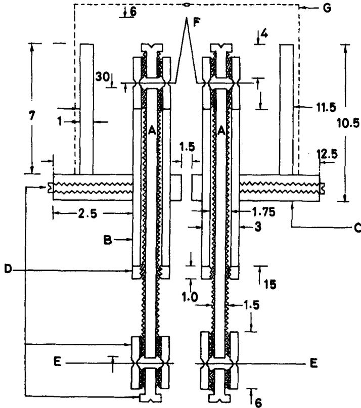
**Figure 2a.** Cross-section view of the replaceable filament-assembly of the high voltage electron gun. A: copper screw; B: ceramic tubing; C: Al-cylinder; D: Brass nut/bolt; E, E: Filament connecting leads; F: Tungsten filament; G: Grid cylinder.
