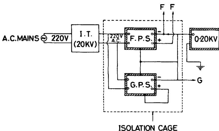
**Figure 3.** Electrical controls for an isolated floating high voltage system. FPS: Filament power supply; GPS: Grid power supply; IT: Isolation transformer; FF: Leads to filament; G: Lead to grid.
