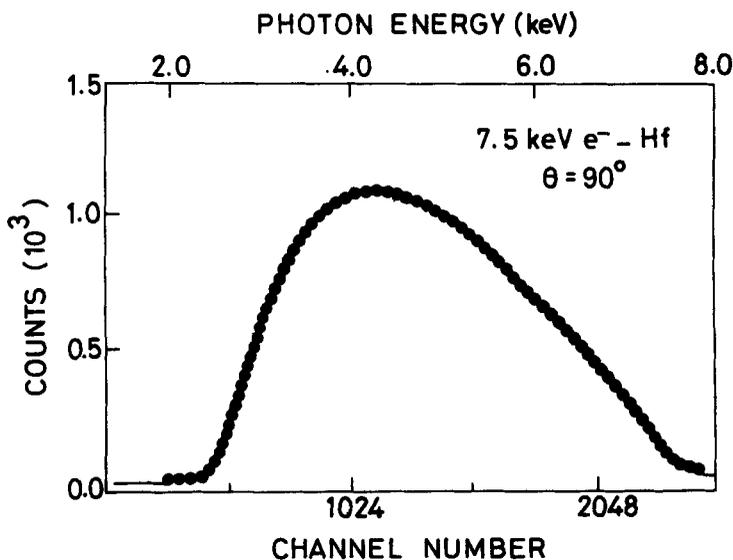
**Figure 5c.** Electron bremsstrahlung photon energy spectrum for 7.5 keV electrons on a thin Hf target.
