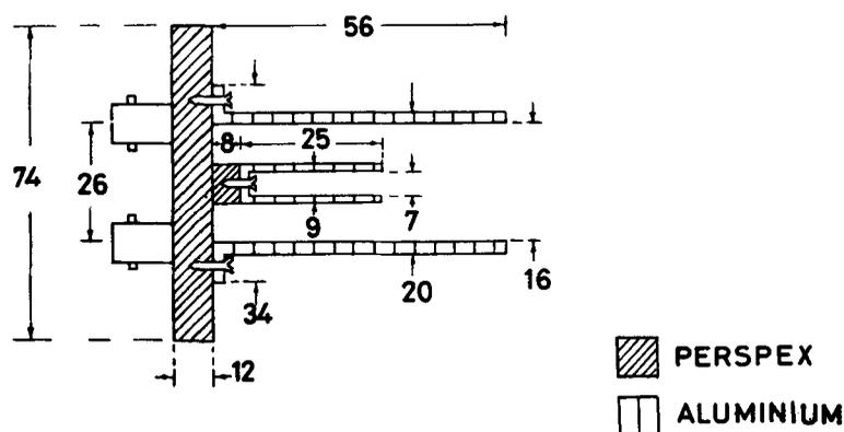
Figure 1b. Cross-section view of the Faraday cup assembly.
