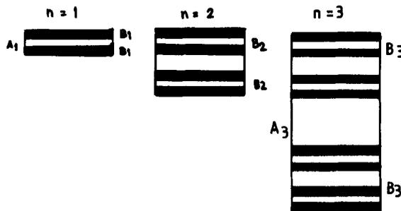
**Figure 1.** Geometry of a cantor bar triadic semiconductor superlattice of one and three generations.
