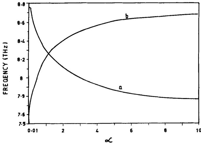
**Figure 5.** Thickness ratio  $\alpha$  as a function of highest GaAs LO frequency of strained CBSSL for three generations with layers A and B as (a)  $(\text{GaSb})_{10}$  and  $(\text{GaAs})_n$ ; (b)  $(\text{GaAs})_{10}$  and  $(\text{GaSb})_n$  respectively.
