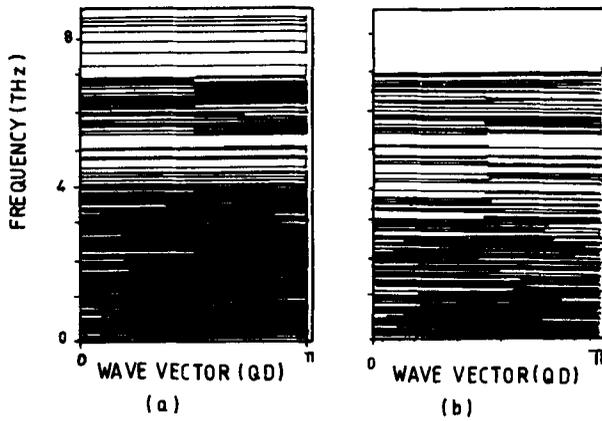
**Figure 4.** Phonon dispersion curves for FSSL of four generations with blocks  $A = (\text{GaSb})_{10}(\text{InAs})_{20}(\text{GaAs})_{10}$ ,  $B = (\text{GaSb})_{10}(\text{InAs})_4(\text{GaAs})_{10}$  for unstrained (a) and strained (b) systems.
