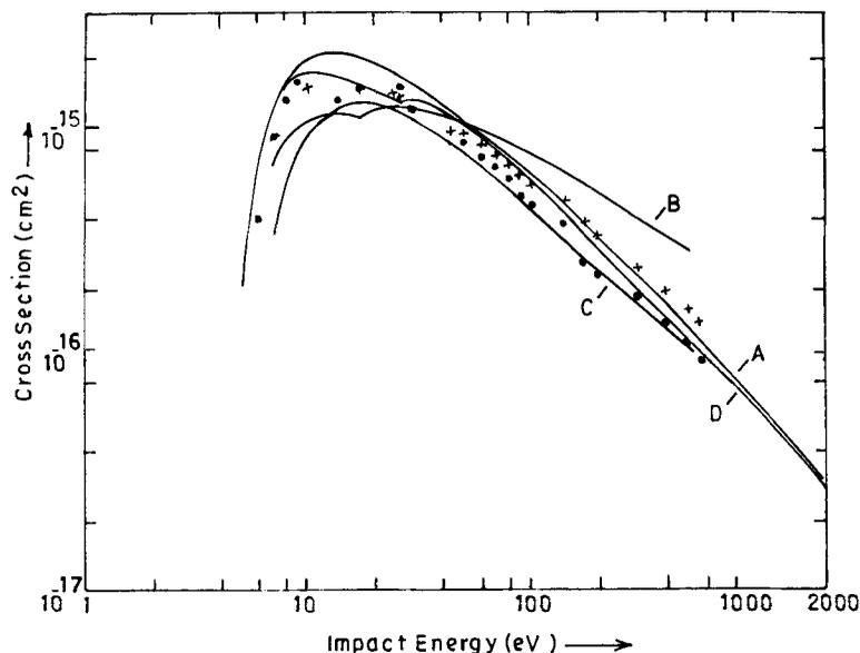
**Figure 1.** Electron impact ionization cross-sections for Ba; (A) Present calculation including contributions from inner shells and excitation-autoionization; (B) Calculation of Lotz [17]; (C) Calculation of McGuire [18]; (D) Present calculation (including contributions from inner shells) excluding excitation-autoionization. (●) Experiment of Dettmann and Karstensen [19]; (×) Experiment of Okudaira [20]
