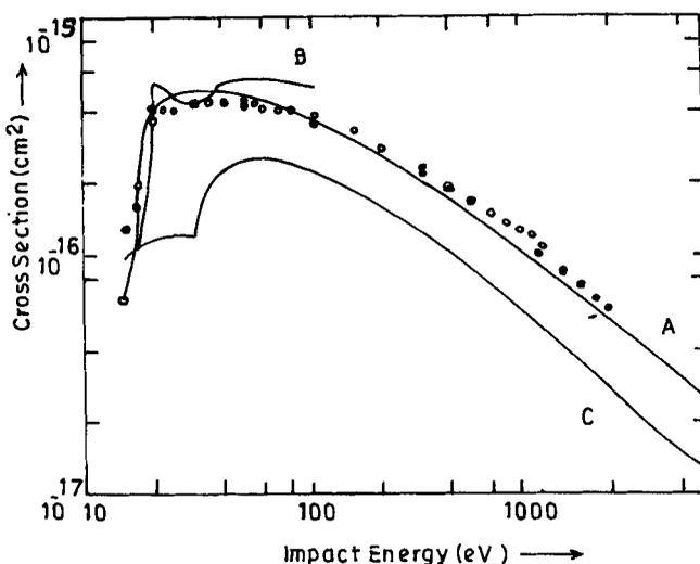
**Figure 2.** Electron impact ionization cross-sections for  $Ba^+$ ; (A) Present calculation including contributions from inner shells and excitation-autoionization; (B) Calculation of Bely *et al* [21]; (C) Present calculation (including contributions from inner shells) excluding excitation-autoionization. (●) Experiment of Peart and Dolder [23]; (○) Experiment of Freney *et al* [24]
