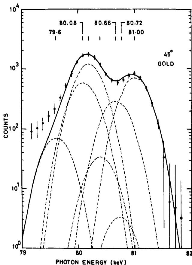
**Figure 3.** Net counts arising at  $45^\circ$  from gold  $K\beta'_2$  X-rays, and elastically scattered 79.6 keV and 81.0 keV  $\gamma$  rays in 40 h. The continuous curve represents the best fit obtained by a least-squares-fitting procedure, the seven dashed curves indicating the corresponding individual contributions as described in § 3. Note the logarithmic scale for counts.
