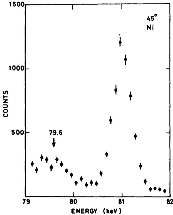
**Figure 2.** Net counts in the neighbourhood of 81 keV obtained at 45° with a nickel target in 9 h. The small peak corresponding to elastic scattering of the weak 79.6 keV  $\gamma$  ray intensity is indicated by an arrow.
