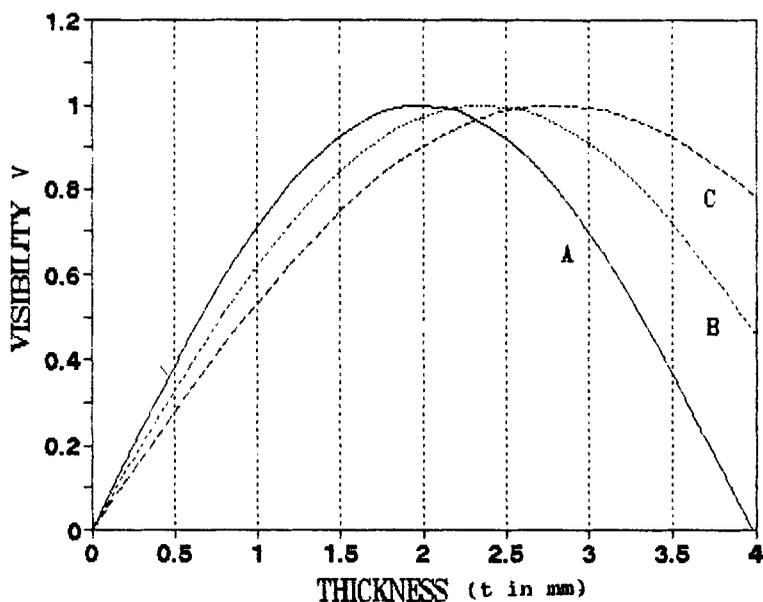
**Figure 4.** Shows the plot between visibility  $V$  and the thickness  $t$  of the BSO crystal for a constant value of  $\lambda = 514$  nm. Curve A,  $\rho = 45^\circ/\text{mm}$ ; curve B,  $\rho = 38^\circ/\text{mm}$  and curve C,  $\rho = 32^\circ/\text{mm}$ .
