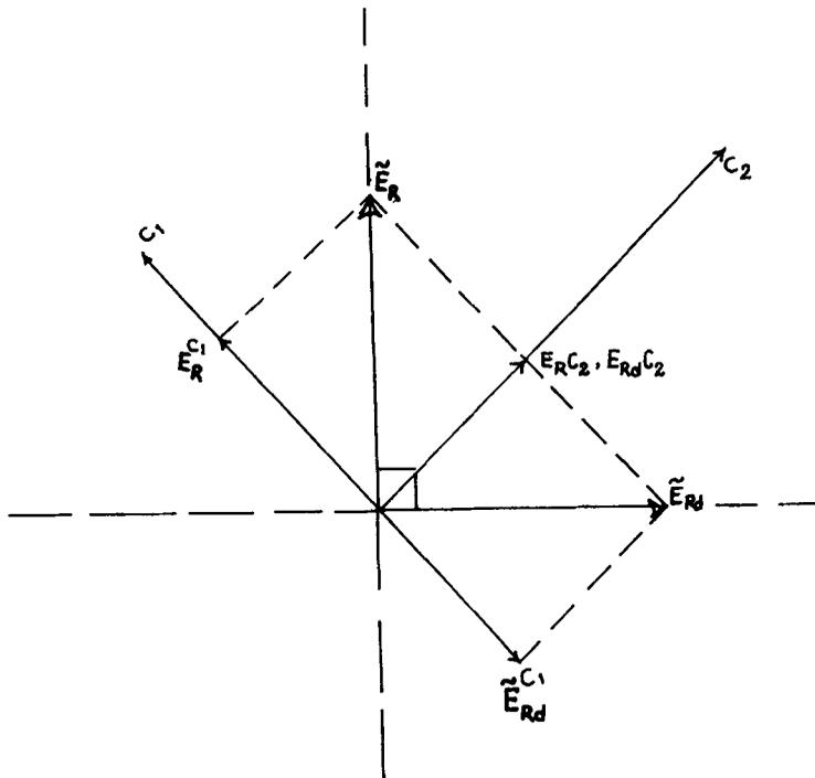
**Figure 3.** Shows the read out mechanism of anisotropic self-diffraction.
