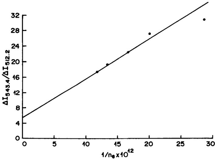
**Figure 4(c).** Variation of the ratio of intensity changes of two spectral lines at 543.4 and 512.2 nm, representing the two states of neon,  $3s_2$  and ( $5s_1'''$  and  $5s_1''$ ) respectively, with respect to the reciprocal of electron density of the plasma in the cell.
