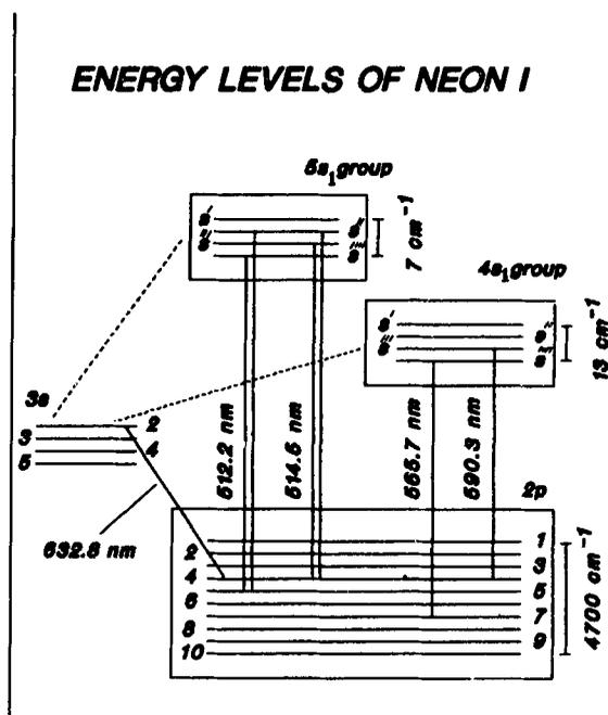
Figure 3. Schematic representation of some of the energy levels of NeI. The energy spacing is only representative and not as per actual values.
