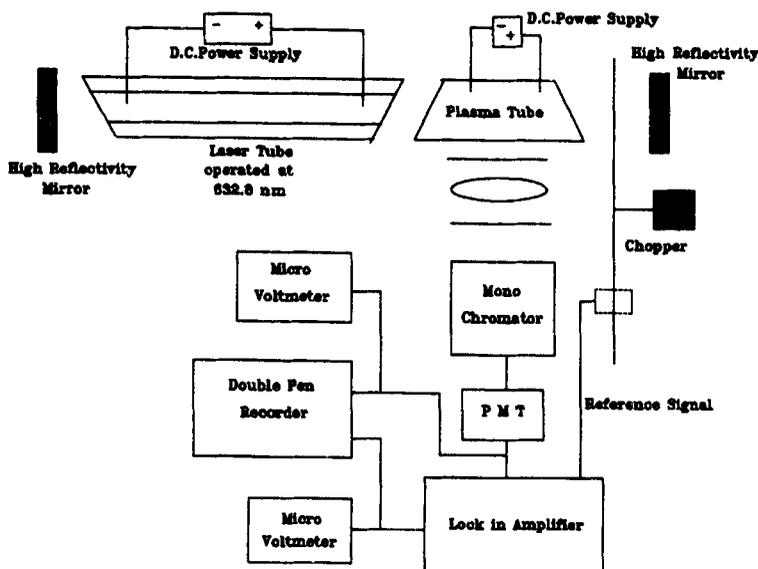
Figure 2. Schematic representation of the experimental set-up.
