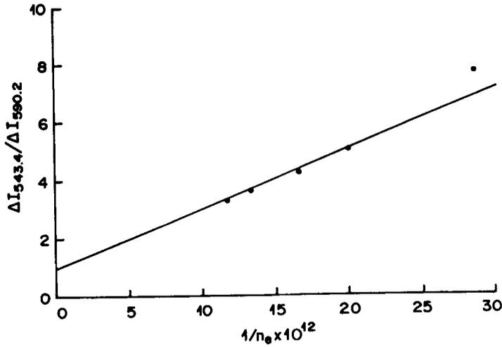
**Figure 4(b).** Variation of the ratio of intensity changes of two spectral lines at 543.4 and 590.2 nm, representing the two states of neon,  $3s_2$  and  $4s_1'''$  respectively, with respect to the reciprocal of electron density of the plasma in the cell.
