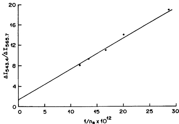
Figure 4(a). Variation of the ratio of intensity changes of two spectral lines at  $543.4$  and  $565.7\text{ nm}$ , representing the two states of neon,  $3s_2$  and  $4s_1'''$  respectively, with respect to the reciprocal of electron density of the plasma in the cell.
