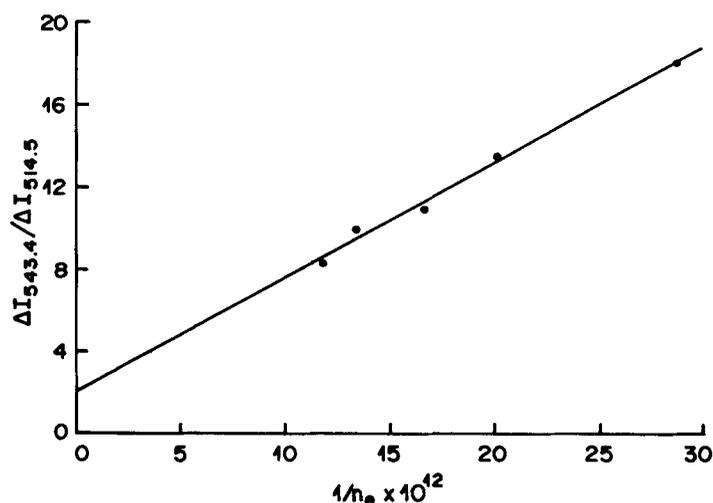
**Figure 4(d).** Variation of the ratio of intensity changes of two spectral lines at 543.4 and 514.5 nm, representing the two states of neon,  $3s_2$  and ( $5s_1'''$  and  $5s_1'$ ) respectively, with respect to the reciprocal of electron density of the plasma in the cell.
