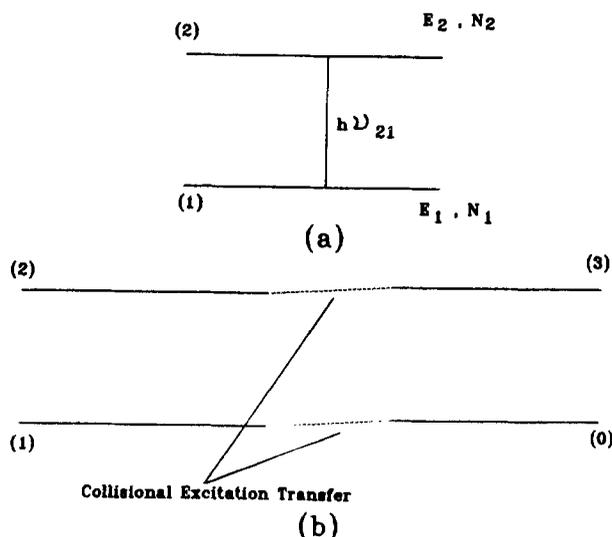
**Figure 1.** Schematic representation of an atomic system with two quantum states (a) (1) and (2) having two more energy states (b) (0) and (3) close to each of them respectively.
