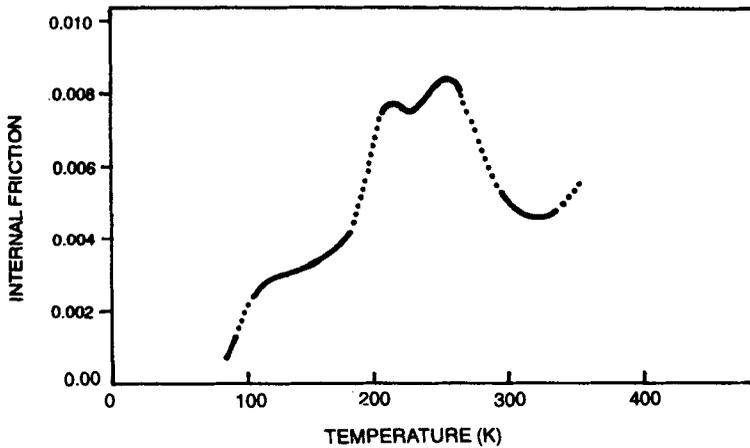
**Figure 4.** Internal friction of the alloy Fe-28 Ni-0.2C during heating from 82 K to 350 K.
