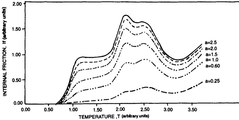
**Figure 3.** Effect of lattice parameter on internal friction temperature behaviour in nonlocal continuum theory.
