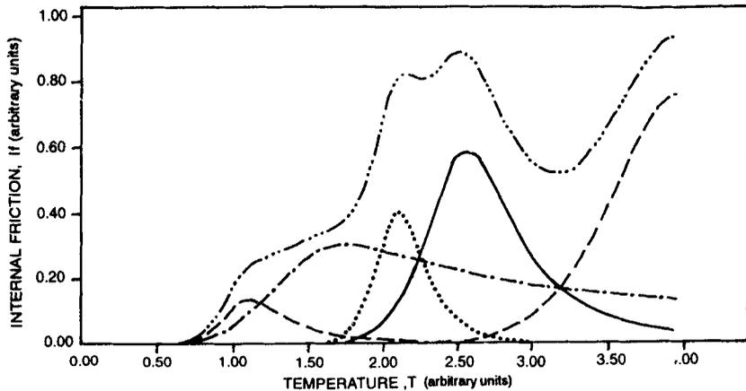
**Figure 2.** Internal friction temperature behaviour in nonlocal continuum theory. Here the lattice parameter is  $a = 0.60$ . Other parameters are kept as constant.
