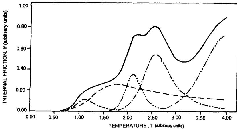
**Figure 1.** Internal friction temperature behaviour in classical continuum theory.
