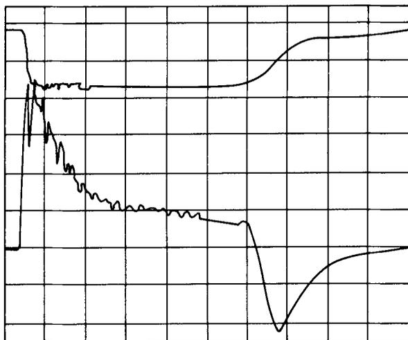
Figure 3. A typical oscilloscope trace for the applied bias (top) and the corresponding current through current transformer (bias). Top trace has y-axis 2000 V/div and x-axis 500 ns/div. Bottom trace has y-axis 100 mA/div and x-axis 500 ns/div. Plasma density  $6.26 \times 10^8$  per cc. Note the current behaviour in the flat top of the applied bias. The model predicts the current in this portion.
