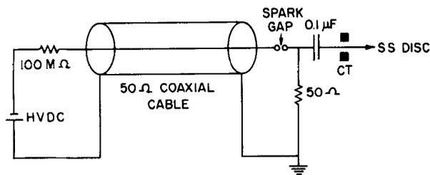
Figure 2. Pulse forming network, CT is the Pearson current transformer.
