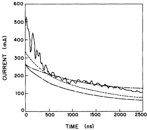
**Figure 4.** Comparison between the current obtained in (i) experiment (—) (ii) the model [Eq. (7)] (---) (iii) conduction current [Eq. (2)] (— · —) (iv) model [Eq. (7)] and contribution from the emitted secondary electrons (----). Applied bias is 3010 V and plasma density is  $9.4 \times 10^8/\text{cc}$ .
