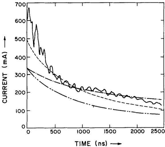
**Figure 5.** Comparison between the current obtained in (i) experiment (—) (ii) the model [Eq. (7)] (---) (iii) conduction current [Eq. (2)] (— · —) (iv) model [Eq. (7)] and contribution from the emitted secondary electrons (----). Applied bias is 4900 V and plasma density is  $9.4 \times 10^8/\text{cc}$ .
