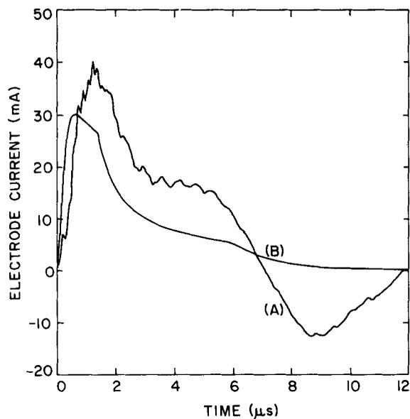
**Figure 6.** Comparison of the experimental [A] and the model current [B].  $n_i = 8.1 \times 10^8 \text{ cc}^{-1}$  and  $\alpha = 0.35$ .
