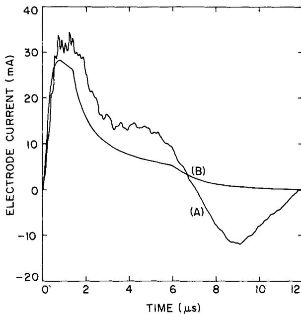
**Figure 5.** Comparison of the experimental [A] and the model current [B].  $n_i = 4.04 \times 10^8 \text{ cc}^{-1}$  and  $\alpha = 0.21$ .
