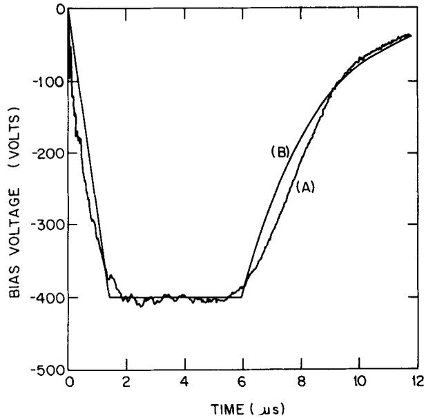
Figure 2. Pulse shapes used in: [A] Experiment [B] Calculation (eq. 15).  $\phi_0 = 400$  V and  $\tau = 2.52$   $\mu$ s.
