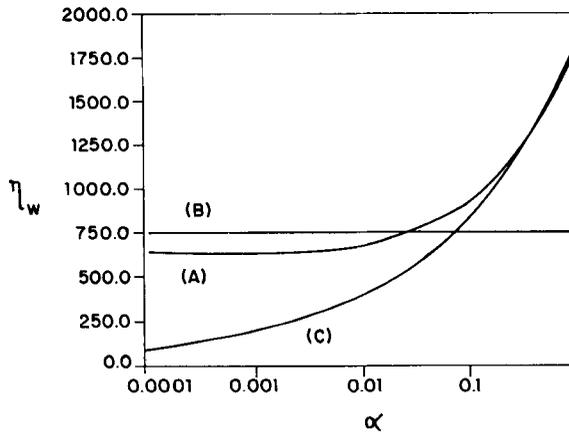
**Figure 4.** Dependence of  $\eta_w$  (dimensionless wall potential) on  $\alpha$  (ratio of debye length to the charge exchange mean free path) for [A] exact equations (eqs 5 and 6) [B] collisionless (eqs 7 and 8) and [C] collisional (eqs 10 and 11). The sheath thickness  $d = 100$  debye lengths.
