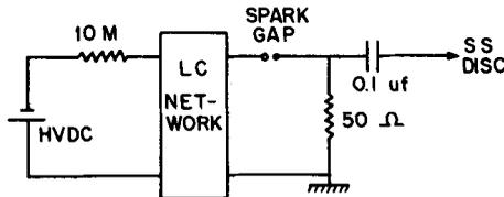
Figure 3. Schematic diagram of the pulse forming circuit.
