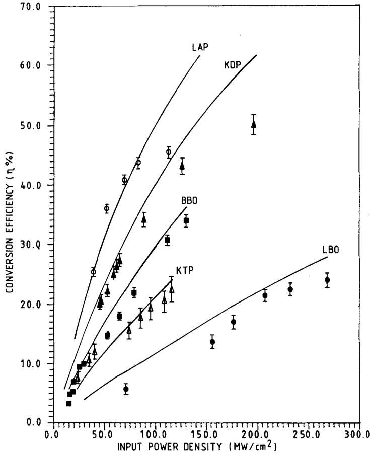
**Figure 2.** Conversion efficiency for SHG in KDP, LAP, KTP, BBO and LBO crystals as a function of the power density of the input Nd:YAG laser pulses. The smooth curves represent the calculated values.
