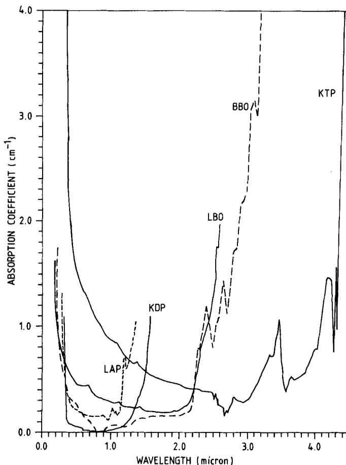
Figure 1. Absorption spectra for 3.5 cm long KDP, 0.7 cm long BBO, 1.6 cm long LAP, 0.5 cm long LBO and 0.5 cm long KTP crystals.
