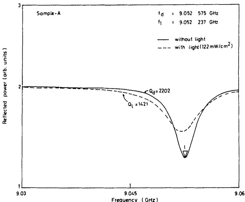
**Figure 10.** Cavity resonance curve for sample-A under dark and under  $122 \text{ mW/cm}^2$  white light illumination.
