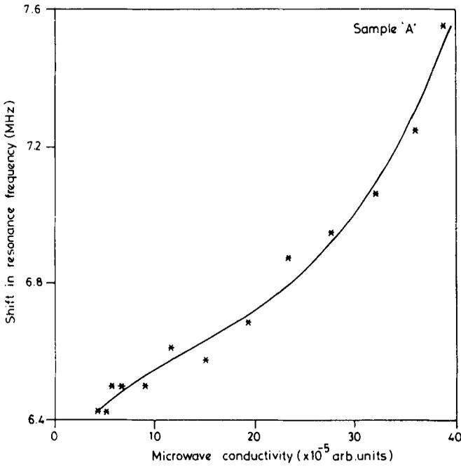
Figure 11. Shift in the resonance frequency with conductivity for sample-A.
