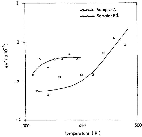
Figure 7. Variation of change in dielectric constant with temperature for samples-A and K1.
