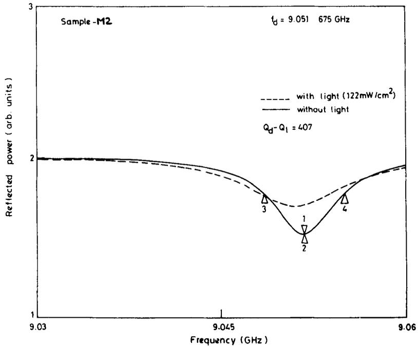
Figure 12. Cavity resonance curve for sample-M2 under dark and under 122 mW/cm<sup>2</sup> white light illumination.
