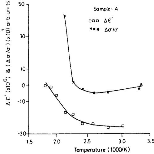
**Figure 9.** Variation of  $\Delta\epsilon'$  ( $\times 10^6$ ) and  $(\Delta\sigma/\sigma)$  ( $\times 10$ ) with temperature for sample-A for comparison.
