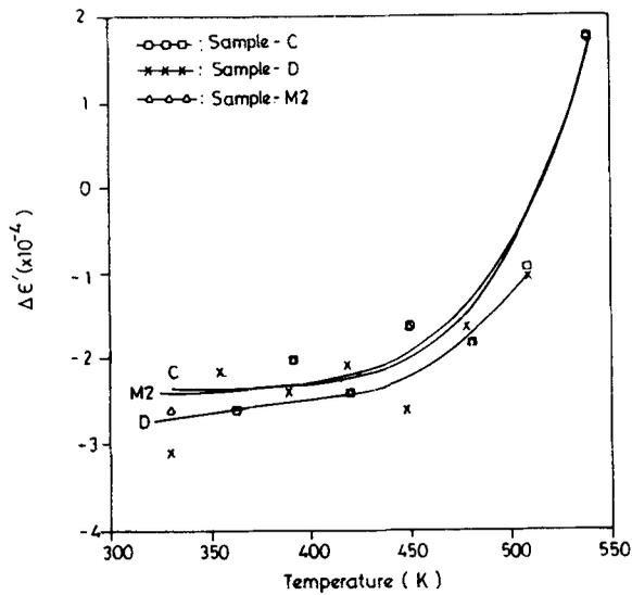
Figure 8. Variation of change in dielectric constant with temperature for samples-C, D, and M2.
