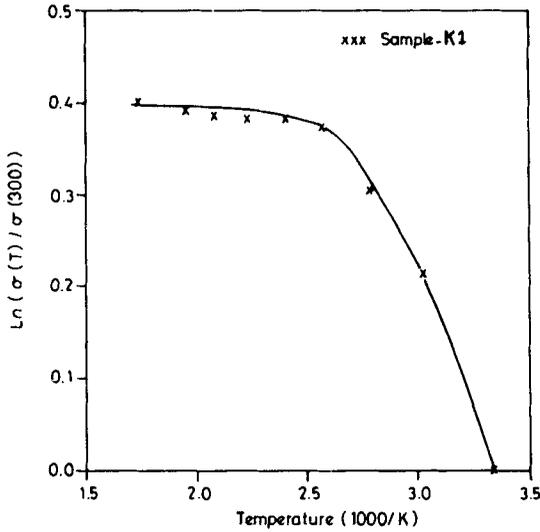
**Figure 6.** Variation of microwave conductivity with temperature for silicon sample-K1. The variation shows that the extrinsic conduction region due to the impurity centre located at 0.28 eV below the conduction band and the subsequent carrier saturation region.
