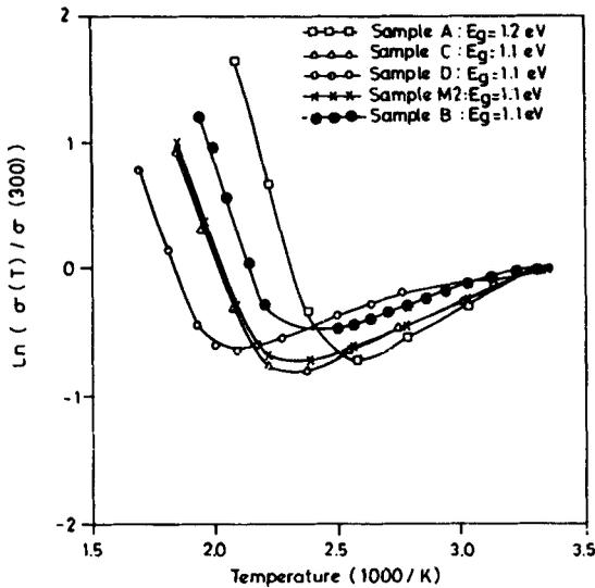
Figure 4. Variation of microwave conductivity with temperature for silicon samples-A, B, C, E, and M2.
