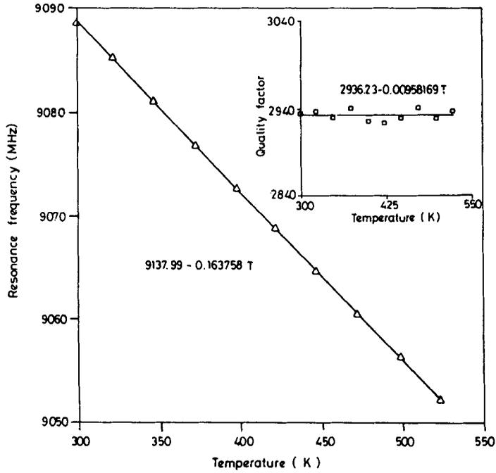
Figure 3. Variation of resonance frequency with temperature. Inset: Variation of quality factor with temperature.
