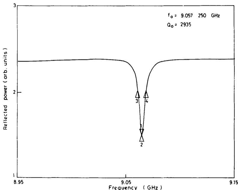
Figure 2. Resonance curve of the empty cavity.
