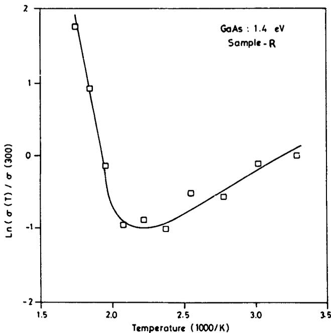
Figure 5. Variation of microwave conductivity with temperature for semi-insulating GaAs sample-R.
