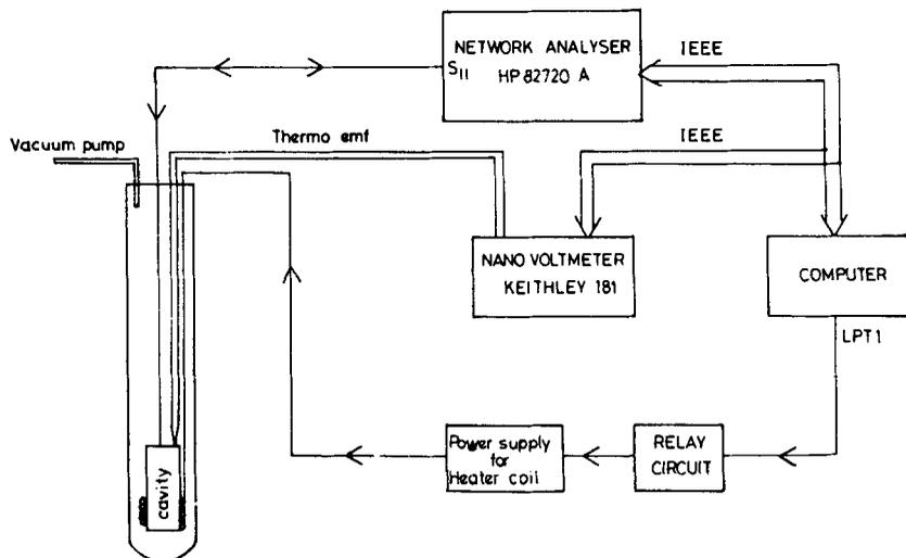
Figure 1. Block diagram of the experimental arrangement to measure the microwave conductivity.
