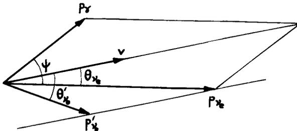
**Figure 2.** Kinematics of the neutrino-photon interaction:  $\mathbf{p}_{\nu_e}$  = linear momentum of the neutrino in the co-ordinate system of the Sun;  $\mathbf{p}_\gamma$  = linear momentum of the photon in the same system;  $\mathbf{v}$  = velocity of the centre of mass (system);  $\mathbf{p}'_{\nu_e}$  = linear momentum of the neutrino in that system.
